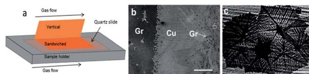
**Fig. 4** (a) Schematics showing the geometrical configuration of the copper foil during typical growth process (bent copper foil), (b) SEM image near the bent region containing both vertical (right) and sandwiched parts (left) and (c) zoomed image of typical graphene islands in the unconfined copper foil. The image in (c) shows the dendritic shape structure due to etching caused by the *in situ* rise in hydrogen partial pressure. The scale bars are (b) 500 μm and (c) 100 μm.
