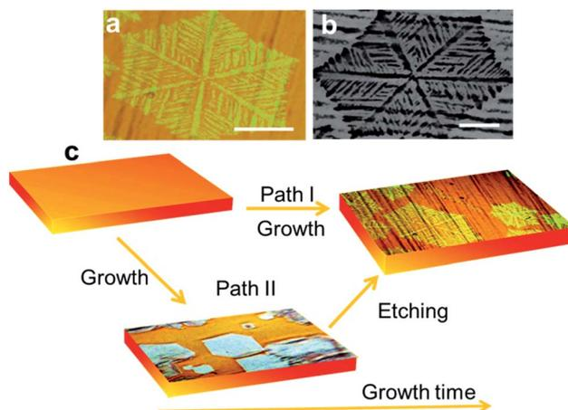
Fig. 1 (a) Optical and (b) SEM picture of as-grown graphene on a copper foil. (c) Scheme showing the two possible pathways leading to the final graphene structure. In prior work, direct growth of dendritic shapes was reported (Path I). We propose that the same structures can be the result of a two-step mechanism (Path II) consisting of growth and subsequent etching. The scale bars are 50  $\mu\text{m}$ .
