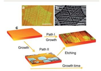
Fig. 1 (a) Optical and (b) SEM picture of as-grown graphene on a copper foil. (c) Scheme showing the two possible pathways leading to the final graphene structure. In prior work, direct growth of dendritic shapes was reported (Path I). We propose that the same structures can be the result of a two-step mechanism (Path II) consisting of growth and subsequent etching. The scale bars are 50 µm.
