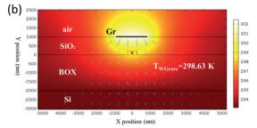
Fig. 4 Simulated thermal field distribution of the proposed structure with graphene contact heating (a) and the conventional structure with 1 μm-thick top SiO<sub>2</sub> cladding layer (b). Blue arrows shows the directions of heat flux
