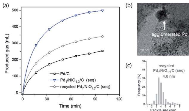
Fig. 8 (a) Catalytic activity test (10 mL 1 M formic acid at 60 °C) over recycled Pd<sub>1</sub>/NiO<sub>1.3</sub>/C (seq) and its (b) TEM images and (c) particle size distribution with average particle size.
