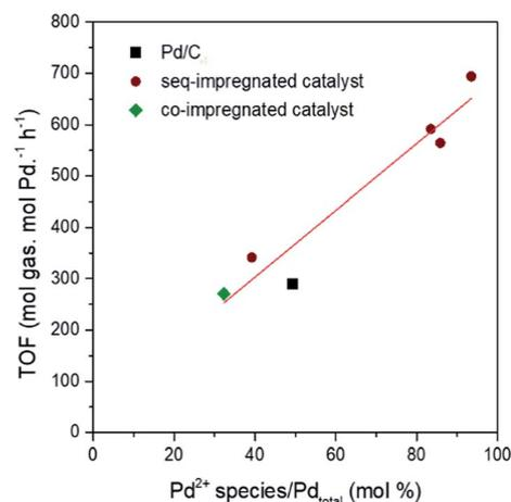
Fig. 7 The correlation between Pd<sup>2+</sup> species/Pd<sub>total</sub> (mol%) and the TOF (mol gas mol Pd<sup>-1</sup> h<sup>-1</sup>) of the catalysts at early 1 min after stabilization (from 3 to 4 min) during the reaction of 10 mL formic acid (1 M) at 60 °C.
