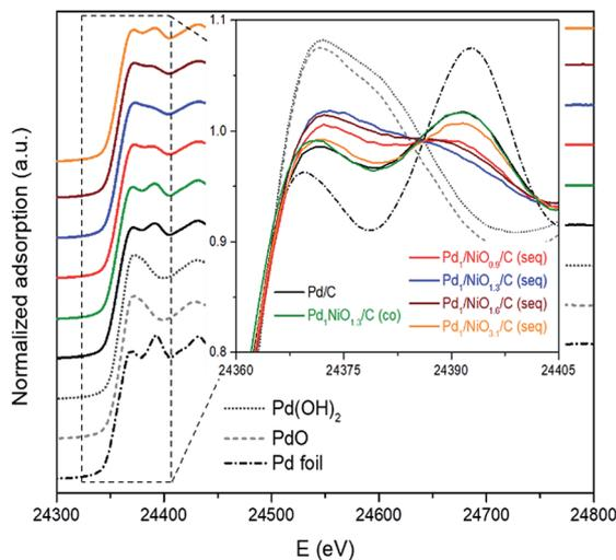
Fig. 5 Normalized XANES spectra for Pd K-edges of Pd–NiO/C catalysts with references (*i.e.* Pd foil, PdO and Pd(OH)<sub>2</sub>).
