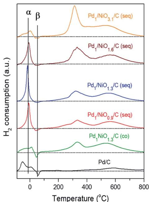
Fig. 6 Cryogenic H<sub>2</sub>-TPR spectra of the various Pd–Ni catalysts obtained after drying.
