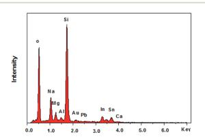
Fig. 6 EDS spectrum of ITO/AuNPs/GSH after incubated in  $10^{-7}$  M Pb<sup>2+</sup> solution.
