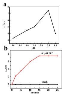
Fig. 7 Effect of pH (a) and time (b) on the wavelength shift of the absorption peaks for the ITO/AuNPs/GSH in the presence of 0.1  $\mu$ M Pb<sup>2+</sup> ions.
