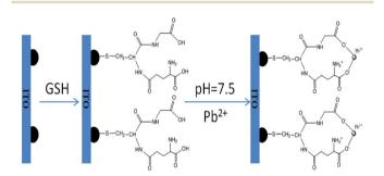
Fig. 5 The mechanism for the LSPR-based detection of Pb2+ ions.
