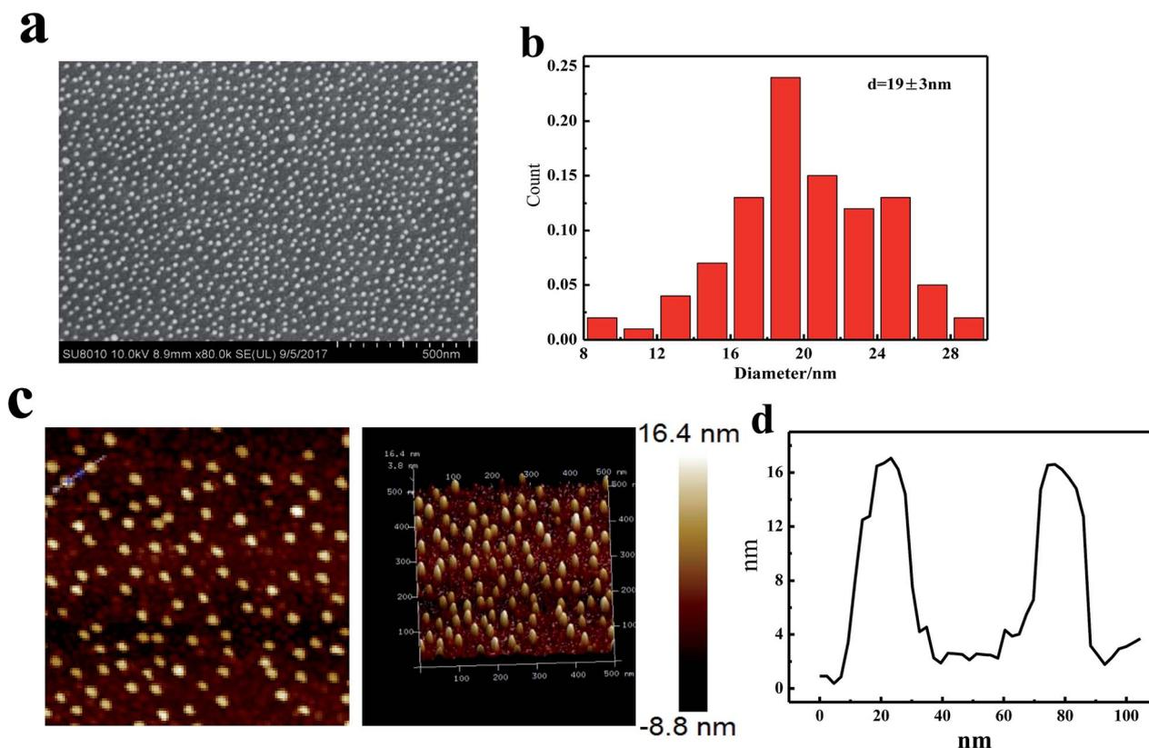
Fig. 2 Typical SEM image of ITO/AuNPs (a), its size distribution (b), AFM scanning images of ITO/AuNPs (c), and its height distribution (d).
