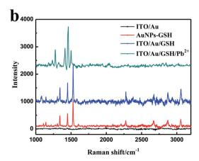
Fig. 4 Cyclic voltammograms of the ITO/AuNPs/GSH and ITO/AuNPs before and after the addition of GSH in a 0.1 M PBS buffer (a), Raman spectra of ITO/AuNPs, AuNPs-GSH, and ITO/AuNPs/GSH before and after the incubation with  $10^{-6}$  M Pb<sup>2+</sup> under a 633 nm excitation in the range of 900-3500 cm<sup>-1</sup> (b).
