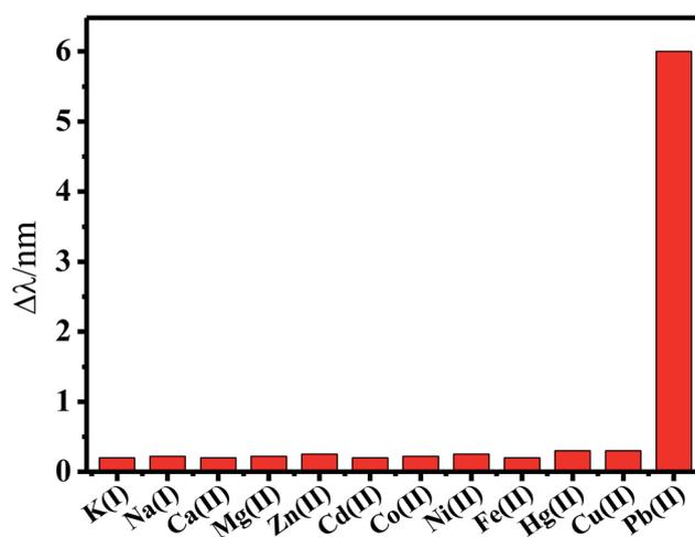
Fig. 9 Comparison of the LSPR peak change for  $\text{Pb}^{2+}$  ions and different metal ions. Concentrations:  $0.01 \mu\text{M}$  for  $\text{Pb}^{2+}$  and  $\text{Cu}^{2+}$  ions,  $1 \mu\text{M}$  for other metal ions.
