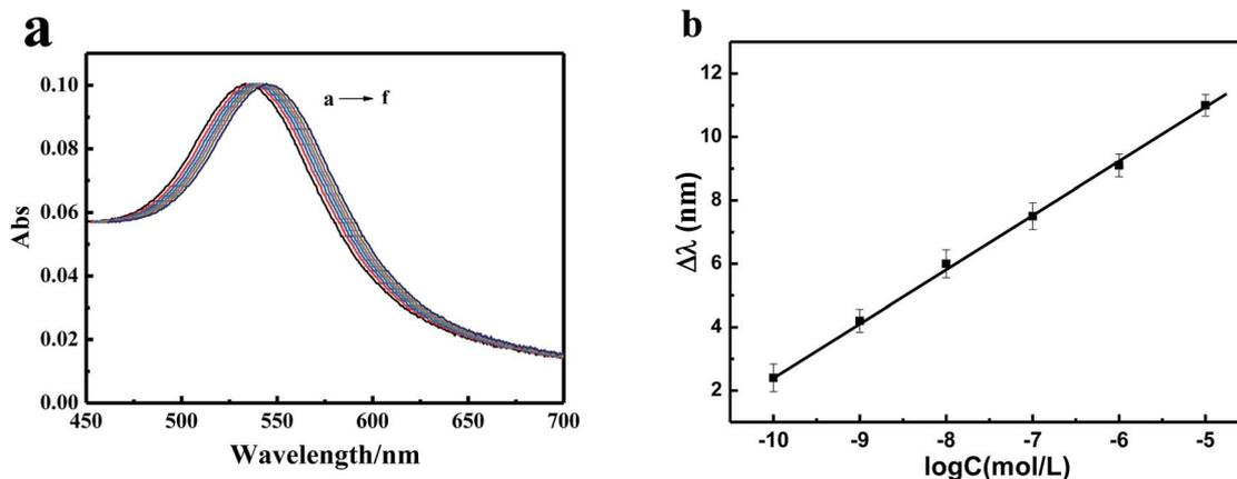
Fig. 8 UV-vis absorption spectra of ITO/AuNPs/GSH in the presence of different concentrations of  $\text{Pb}^{2+}$  (from a to f): 0,  $10^{-10}$ ,  $10^{-9}$ ,  $10^{-8}$ ,  $10^{-7}$ ,  $10^{-6}$ , and  $10^{-5}$  M, respectively (a) and the linear calibration curve between the red-shift of the peak and the concentrations of  $\text{Pb}^{2+}$  (b). Each error bar represents the standard deviation of three measurements.
