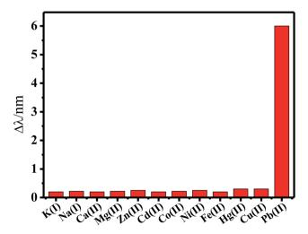
Fig. 9 Comparison of the LSPR peak change for Pb<sup>2+</sup> ions and different metal ions. Concentrations:  $0.01\,\mu\text{M}$  for Pb<sup>2+</sup> and Cu<sup>2+</sup> ions, 1  $\mu\text{M}$  for other metal ions.
