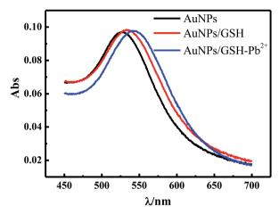
Fig. 3 UV-visible absorption spectra of the ITO/AuNPs and ITO/AuNPs/GSH before and after the incubation with  $10^{-7}$  M Pb<sup>2+</sup> in a Tris–HCl buffer solution.
