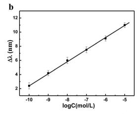
Fig. 8 UV-vis absorption spectra of ITO/AuNPs/GSH in the presence of different concentrations of Pb $^{2+}$  (from a to f): 0,  $10^{-10}$ ,  $10^{-9}$ ,  $10^{-8}$ ,  $10^{-7}$ ,  $10^{-6}$ , and  $10^{-5}$  M, respectively (a) and the linear calibration curve between the red-shift of the peak and the concentrations of Pb $^{2+}$  (b). Each error bar represents the standard deviation of three measurements.
