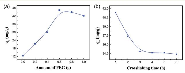
Fig. 2 Effect of the amount of PEG (a) and the crosslinking time (b) for the PCMC bead adsorption of Co(ii).
