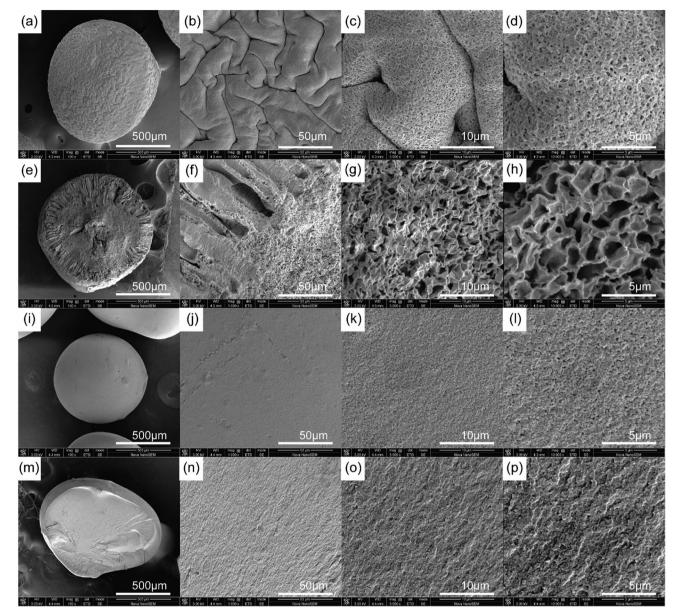
Fig. 5 SEM images of a PCMC bead (a-d) and its cross-section (e-h), and a CMC bead (i-l) and its cross-section (m-p) at  $100\times$ ,  $1000\times$ ,  $1000\times$ , and  $10000\times$  magnification, respectively.
