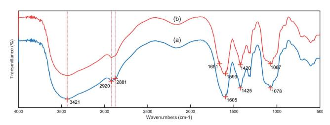
Fig. 4 IR spectra of the CMC (a) and PCMC (b) beads.
