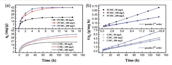
Fig. 11 (a) Effect of contact time on the adsorption capacity of the PCMC and CMC beads at different initial concentrations and (b) the kinetic curves (fitting to the pseudo-second order equation) for the adsorption of Co(II) onto the PCMC and CMC beads.
