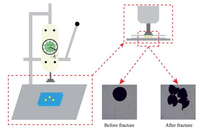
Fig. 3 Schematic diagram of mechanical strength measurements.
