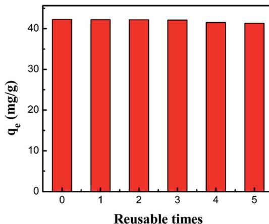
Fig. 17 Regeneration of the PCMC beads (0.05 g adsorbent, 25 mL 200 mg L<sup>-1</sup> cobalt solution, pH 6.0).
