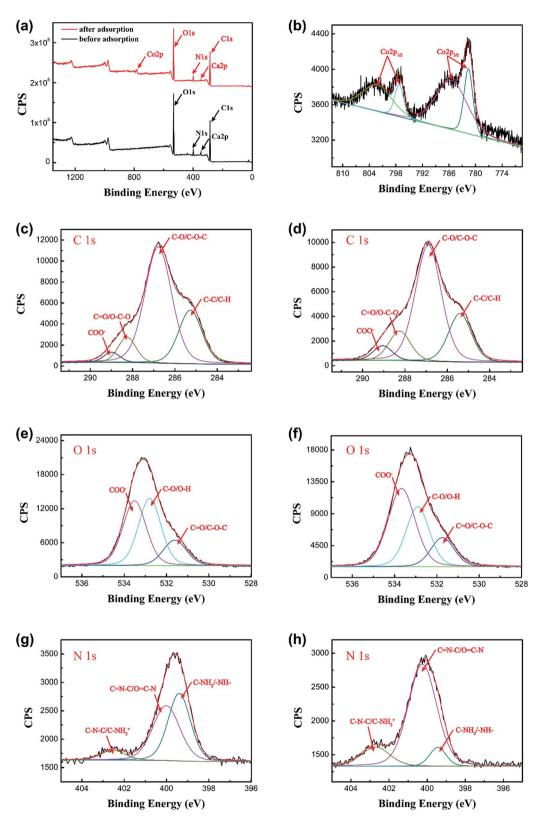
Fig. 15 (a) XPS spectra for the PCMC beads before and after Co(II) adsorption, and (b) the Co 2p spectrum of the PCMC beads after Co(II) adsorption. XPS spectra of C 1s, O 1s and N 1s before ((c), (e), and (g)) and after ((d), (f), and (h)) Co(II) adsorption of the PCMC beads.
