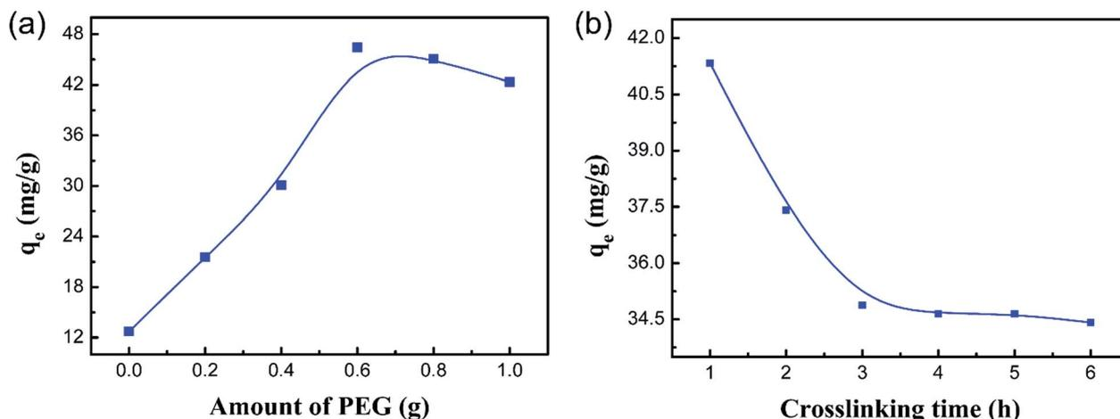
Fig. 2 Effect of the amount of PEG (a) and the crosslinking time (b) for the PCMC bead adsorption of Co(II).
