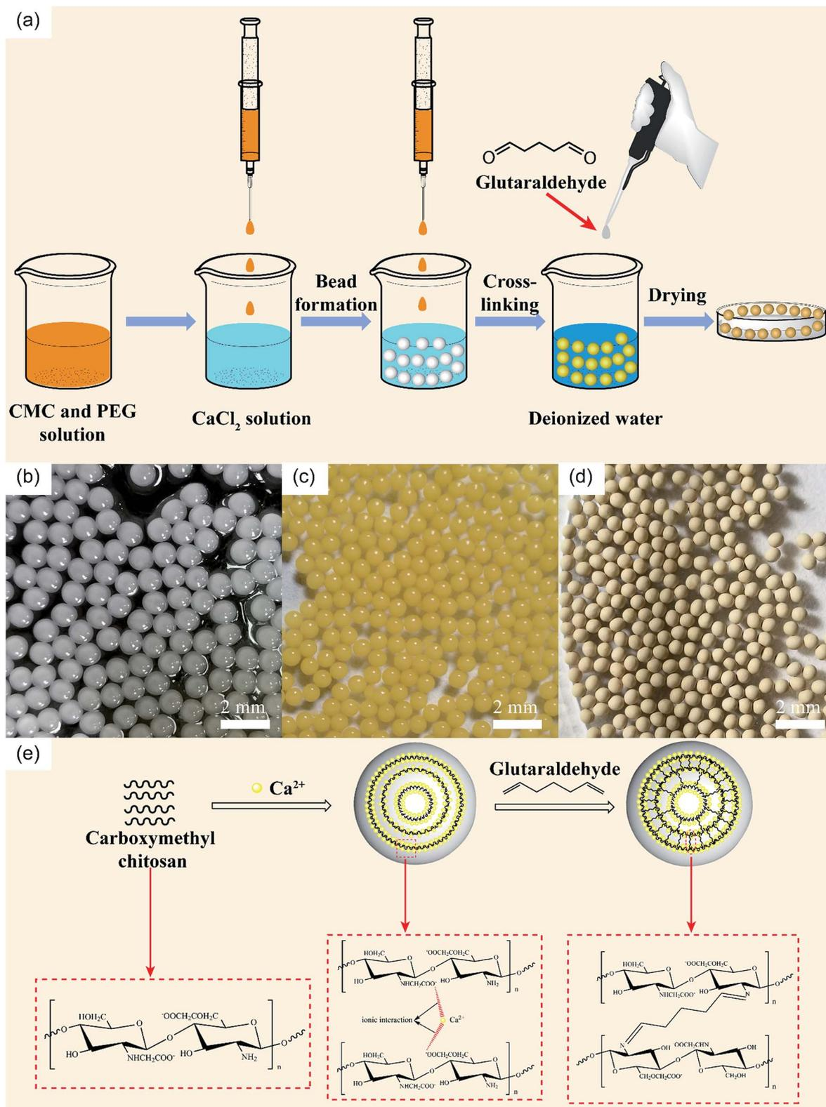
Fig. 1 (a) Schematic illustration of the preparation of PCMC beads. Photos of CaCl<sub>2</sub> physical-crosslinking beads (b), glutaraldehyde chemical-crosslinking beads (c), and beads after drying (d). (e) Mechanism of PCMC beads formation.
