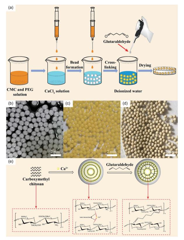
Fig. 1 (a) Schematic illustration of the preparation of PCMC beads. Photos of CaCl<sub>2</sub> physical-crosslinking beads (b), glutaraldehyde chemicalcrosslinking beads (c), and beads after drying (d). (e) Mechanism of PCMC beads formation.
