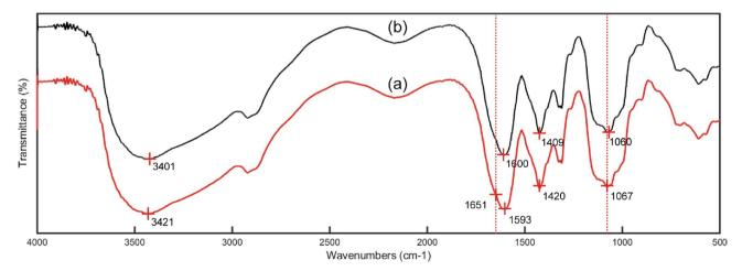
Fig. 14 FTIR spectra of the PCMC beads before (a) and after (b) Co(II) adsorption.
