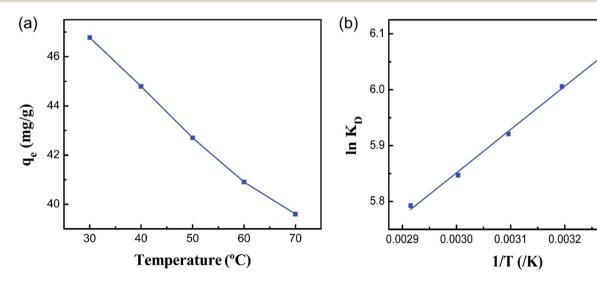
Fig. 10 (a) Effect of temperature on the adsorption capacity of the PCMC beads for Co( $\shortparallel$ ) and (b) the relationship between ln  $K_D$  and 1/T for Co( $\shortparallel$ ) adsorption of the PCMC beads.
