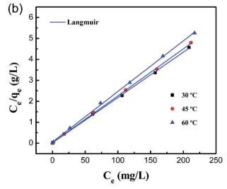
Fig. 12 (a) Effect of the initial concentration on the adsorption capacity of the PCMC beads for Co(ii) and (b) the Langmuir model for the adsorption of Co(II) on the PCMC beads.
