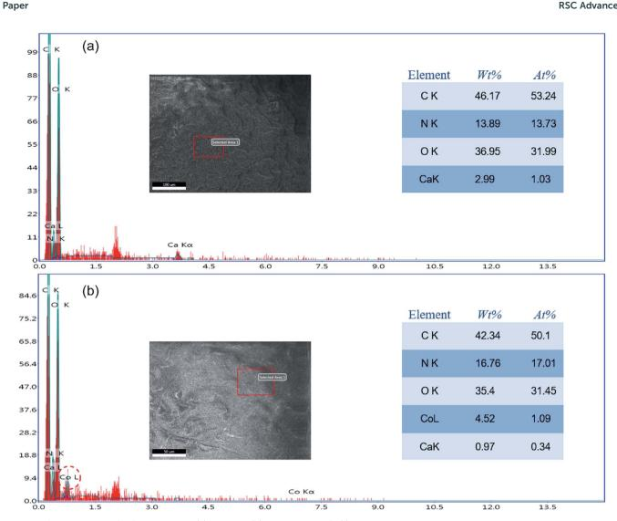
EDS spectra of a PCMC bead before (a) and after (b) adsorption of Co(II).
