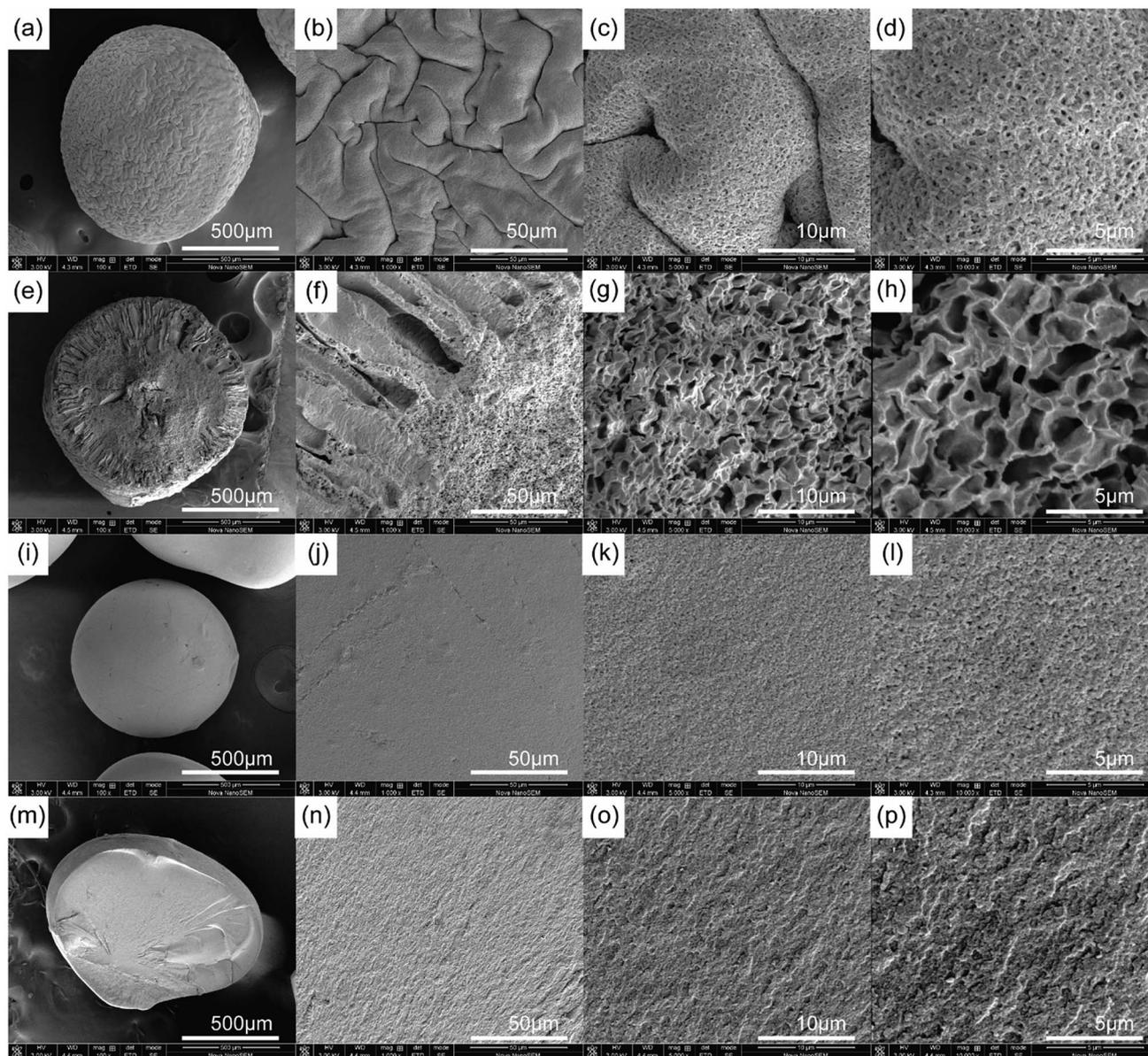
Fig. 5 SEM images of a PCMC bead (a–d) and its cross-section (e–h), and a CMC bead (i–l) and its cross-section (m–p) at 100 $\times$ , 1000 $\times$ , 5000 $\times$ , and 10000 $\times$  magnification, respectively.
