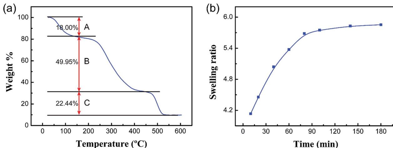
Fig. 7 (a) TGA curve of the PCMC beads and (b) the swelling ratios of the PCMC beads with contact time in the experimental solution.
