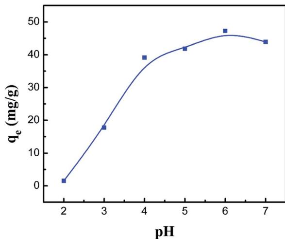
Fig. 9 Effect of the pH value on the adsorption capacity of the PCMC beads.
