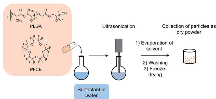
Fig. 1 Schematic representation of miniemulsion formulation method. PLGA and PFCE are added to surfactant solution under sonication, followed by solvent evaporation. Next, particles are washed, freeze-dried, and collected as a dry powder.
