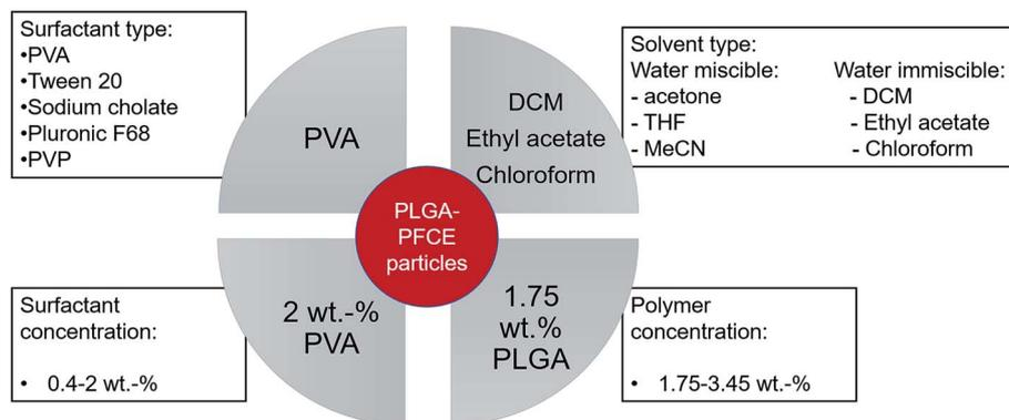
**Scheme 1** Schematic representation of parameters, which affect properties of nanoparticles, tested in this study, including factors that resulted in nanoparticles with low PDI, narrow size distribution and high PFCE content.
