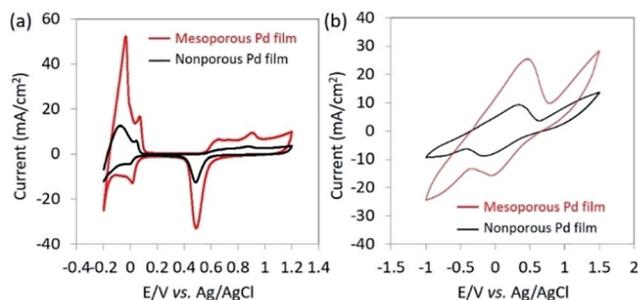
Fig. 2 (a) CV curves of bare mesoporous Pd film and bare nonporous Pd films measured in 0.5 M H<sub>2</sub>SO<sub>4</sub> solution at a scan rate of 50 mV s<sup>-1</sup>. (b) CV curves of bare mesoporous Pd film and bare nonporous Pd films measured in 0.4% NaCl solution containing lactic acid (10 mM). The currents are normalized by the geometric electrode area.
