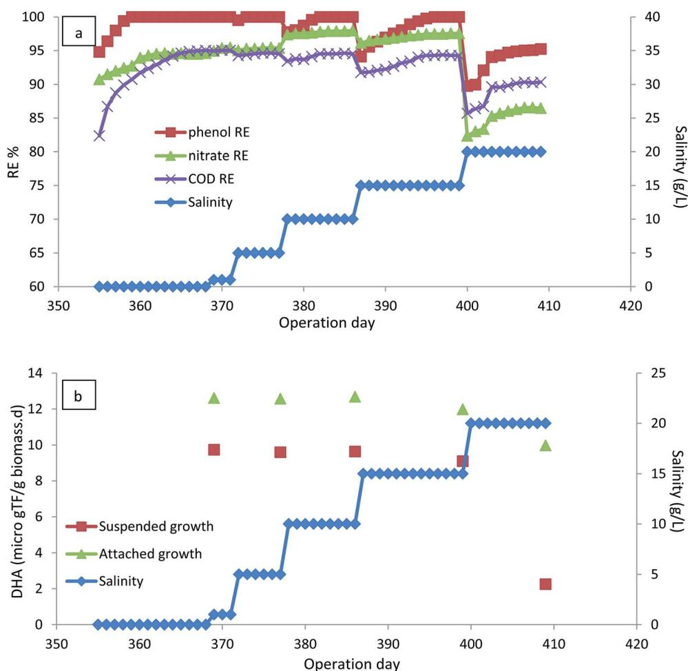
Fig. 6 (a) The effect of salinity on the performance of the CASIR bioreactor. (b) The effect of salinity on the DHA of biomass and biofilm. (HRT = 24 h, inlet phenol concentration =  $500 \text{ mg L}^{-1}$ , MLSS =  $4000 \text{ mg L}^{-1}$ ).
