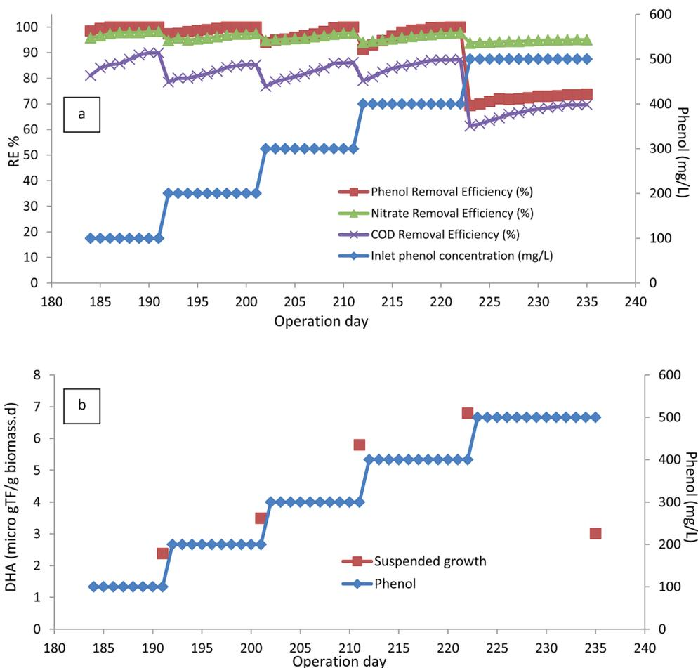
Fig. 4 (a) Performance of the bioreactor without the presence of media. (b) DHA of the bioreactor without the presence of media. (HRT = 24 h, media filling ratio = 0%, MLSS = 4000 mg L<sup>-1</sup>).
