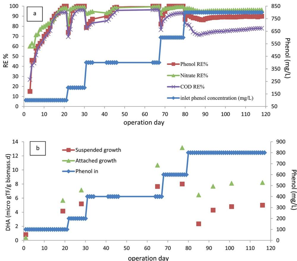
Fig. 2 (a) Start-up and the effect of inlet phenol concentration on phenol, COD and nitrate removal. (b) Variation of DHA within the start-up stage and varying inlet phenol concentration. (HRT = 24 h, media filling ratio = 40%, MLSS = 4000 mg L<sup>-1</sup>).
