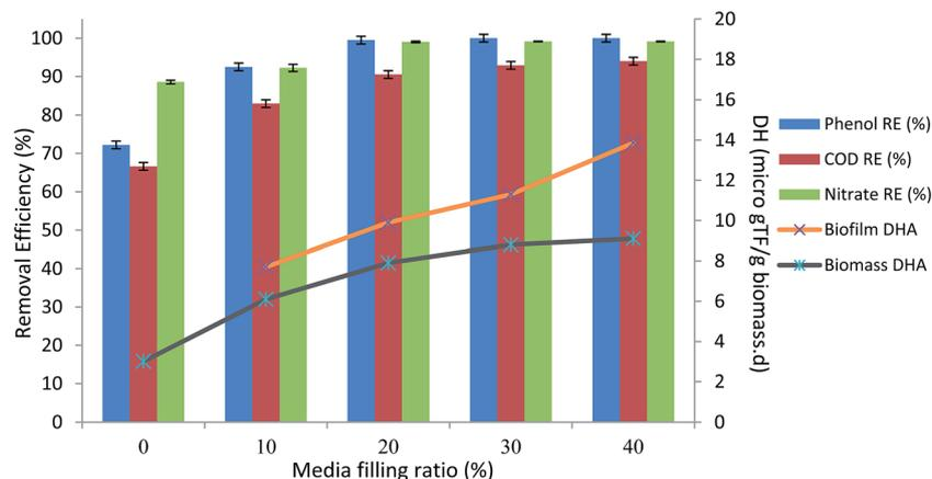
Fig. 5 Average steady-state phenol, COD, nitrate reduction and DHA variation in various media filling ratios. (HRT = 24 h, inlet phenol concentration = 500 mg L<sup>-1</sup>, MLSS = 4000 mg L<sup>-1</sup>).
