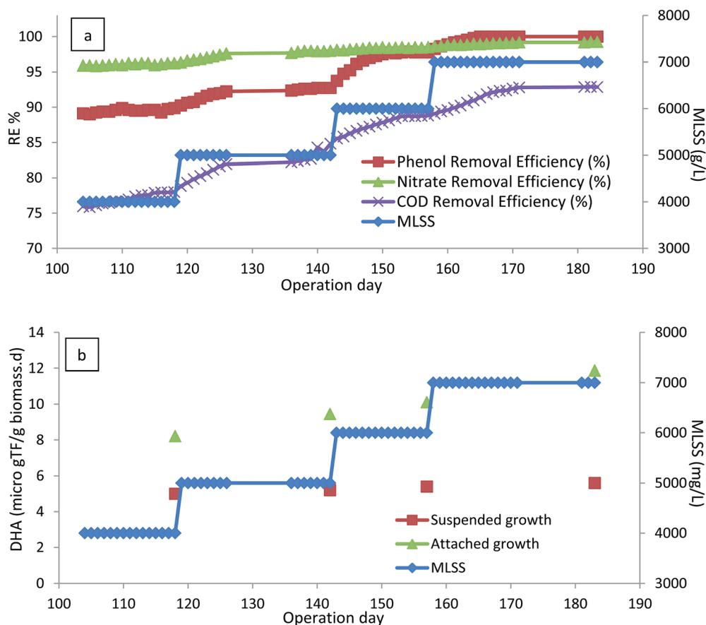
Fig. 3 (a) Effect of MLSS on the performance of the bioreactor. (b) Variation of DHA as a function of MLSS. (HRT = 24 h, media filling ratio = 40%, inlet phenol concentration = 800 mg L<sup>-1</sup>).
