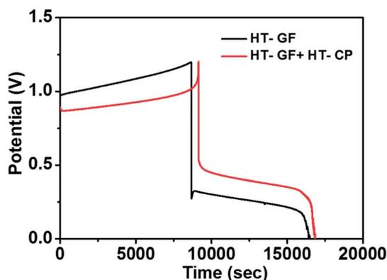
Fig. 6 Charge–discharge curves of Fe/Cu RFB cells with HT-GF and HT-GF + HT-CP at a current density of 20 mA cm<sup>-2</sup>.
