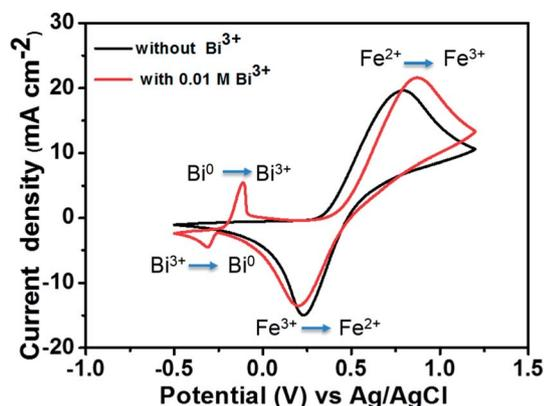
Fig. 4 CV curves of 1.5 M FeCl<sub>2</sub> in a 3 M HCl using GC electrode with and without 0.01 M Bi<sup>3+</sup> at a scan rate of 50 mV s<sup>-1</sup>.
