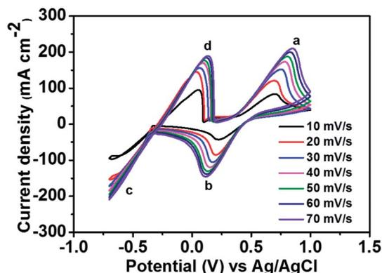
Fig. 3 CV curves of 1.8 M CuCl in a mixed supporting electrolyte (2.4 M CaCl<sub>2</sub> + 2.4 M HCl) solution using GC electrode at various scan rates.
