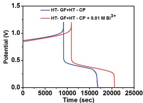
Fig. 7 Charge-discharge curves of a Fe/Cu RFB with and without 0.01 M Bi<sup>3+</sup> in the electrolytes at a current density of 20 mA cm<sup>-2</sup>.
