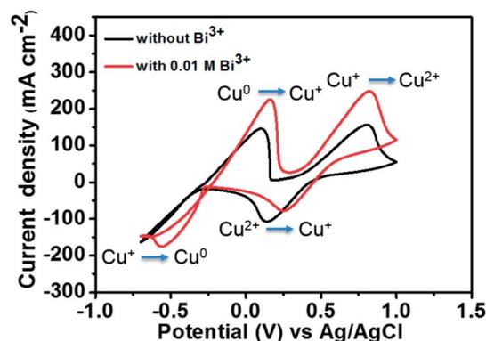
Fig. 5 CV curves of 1.8 M CuCl in a mixed supporting electrolyte (2.4 M CaCl<sub>2</sub> + 2.4 M HCl) solution using GC electrode with and without 0.01 M Bi<sup>3+</sup> at a scan rate of 50 mV s<sup>-1</sup>.
