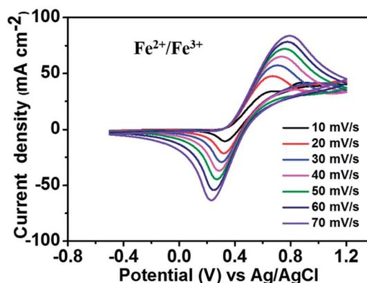
Fig. 2 CV curves of 1.5 M FeCl<sub>2</sub> in a 3 M HCl using GC electrode at various scan rates.
