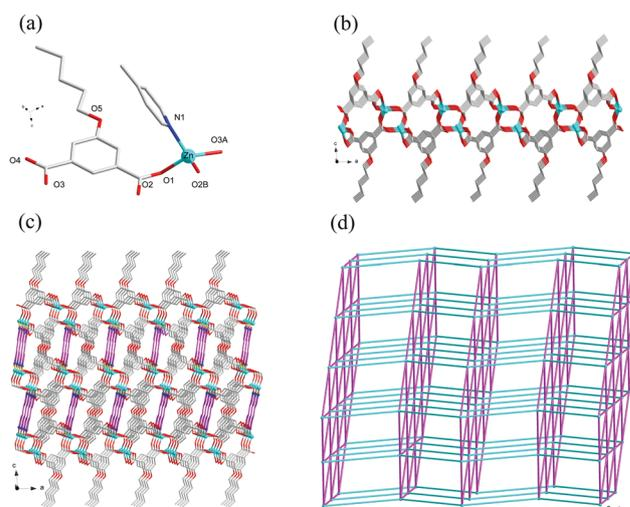
Fig. 7 (a) Coordination environment of the Zn(II) centers in 8 with the hydrogen atoms omitted for clarity (symmetric codes: (A)  $x + 1/2, y - 1/2, z$  and (B)  $-x, y, -z + 1/2$ ). (b) The 2D layer constructed from  $^n$ PeOip ligands and Zn(II) ions. (c) View of the 3D  $[Zn(^n$ PeOip)(bpe)] $_n$  coordination network of 8. (d) View of the topological net of 8.
