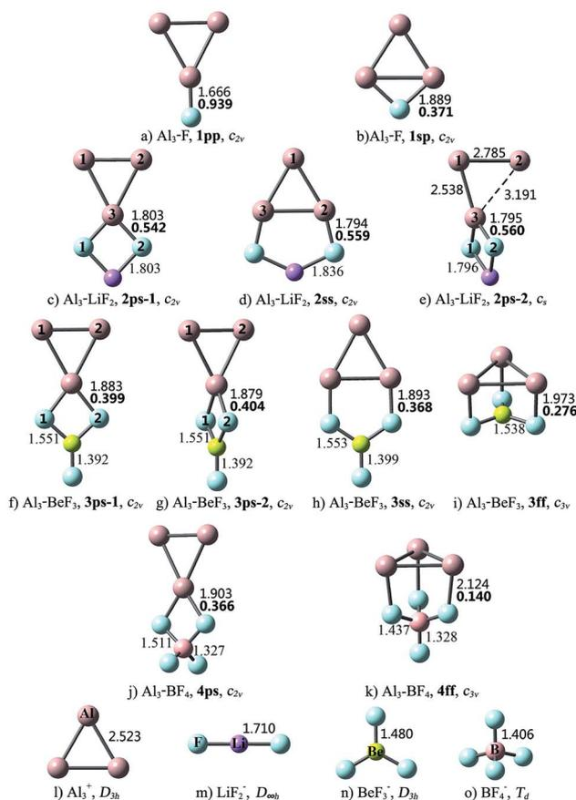
Fig. 1 Optimized structures of the Al<sub>3</sub>-X compounds and Al<sub>3</sub><sup>+</sup>, LiF<sub>2</sub><sup>-</sup>, BeF<sub>3</sub><sup>-</sup>, BF<sub>4</sub><sup>-</sup> ions at the MP2/6-311+G(3df) level, bond lengths (Å) and Laplacian of the electron density at a bond critical point  $\nabla^2\rho(r)$  (in au., bold font) for the Al–F bonds that connect Al<sub>3</sub> and X subunits.
