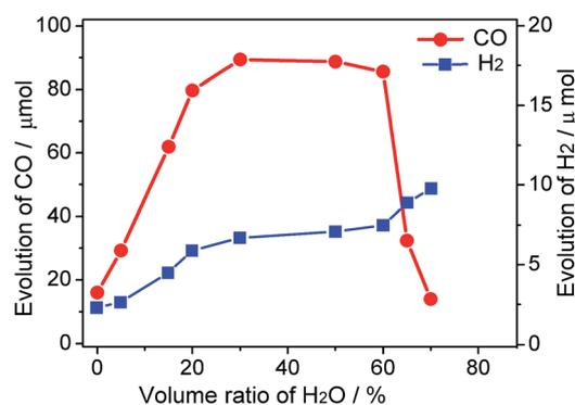
Fig. 1 Effect of the water concentration on the evolution of CO/H<sub>2</sub> in H<sub>2</sub>O–MeCN system.
