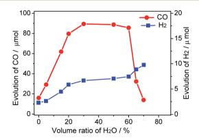
Fig. 1  $\,$  Effect of the water concentration on the evolution of CO/H $_2$  in H $_2\text{O}-\text{MeCN}$  system.
