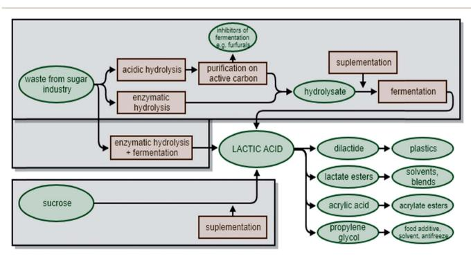
Fig. 3 Usage of sugars derived from biomass and crystalline sucrose in lactic acid production.
