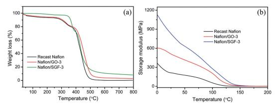
Fig. 6 (a) TGA and (b) DMA curves of pristine recast Nafion and composite membranes.
