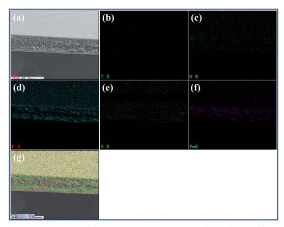
Fig. 4 (a) SEM image of selected area of Nafion/SGF-3; corresponding elemental mappings of (b) carbon, (c) oxygen, (d) fluorine, (e) sulfur, (f) iron and (g) overlapping of elements.
