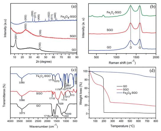
Fig. 2 (a) XRD patterns, (b) Raman spectra, (c) FT-IR spectra and (d) TGA curves of GO, SGO and Fe<sub>3</sub>O<sub>4</sub>-SGO.
