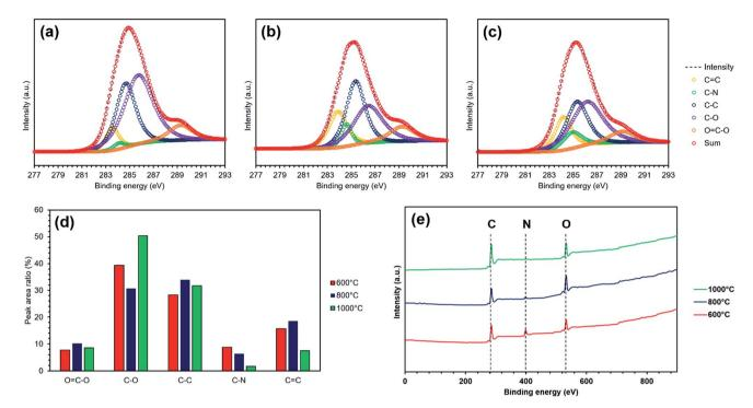
Fig. 5 XPS narrow spectra of the junction-less 3DCS carbonized at (a)  $600 \,^{\circ}$ C, (b)  $800 \,^{\circ}$ C, and (c)  $1000 \,^{\circ}$ C. (d) Functional group component ratio of the junction-less 3DCS carbonized at (red)  $600 \,^{\circ}$ C, (blue)  $800 \,^{\circ}$ C, and (green)  $1000 \,^{\circ}$ C. (e) XPS wide spectra of the junction-less 3DCS carbonized at (red)  $600 \,^{\circ}$ C, (blue)  $800 \,^{\circ}$ C, and (green)  $1000 \,^{\circ}$ C.
