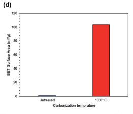
Fig. 2 (a) FE-SEM images of the melamine sponge (a) (Left) before carbonization (Right) after carbonization at 1000 °C, (b) fibre diameter histogram of the melamine sponge (blue) before carbonization (red) after carbonization at 1000 °C and, (c) resistance of the melamine sponge at various carbonization temperatures. (d) BET surface area of the melamine sponge (blue) before carbonization (red) after carbonization at 1000 °C
