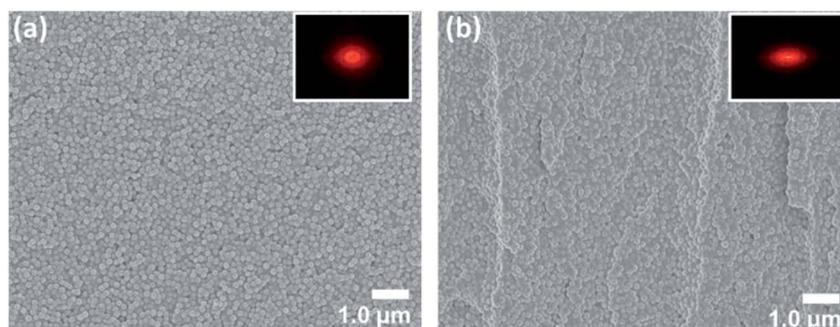
Fig. 3 (a) Top surface and (b) cross-section of FESEM images of the AR structurally colored contact lenses with  $\phi_{\text{silica}} = 30\%$  (sample C). Inset shows the 2D FFT images that exhibited long-range disordered and short-range ordered structures.
