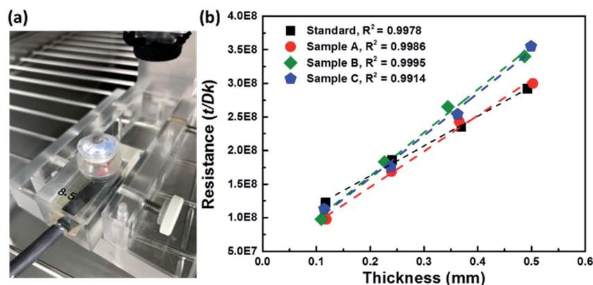
Fig. 6 (a) Polarographic electrode cell for measuring the Dk of sample C. (b) Corrected resistance versus thickness plots for all contact lens samples. The plots are closely approximated by a line ( $R^2 > 0.99$ ).
