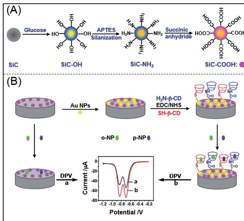
**Scheme 1** The illustration of electrochemical sensing strategy for nitrophenol isomers based on  $\beta$ -cyclodextrin derivatives functionalized silicon carbide. (A) Synthesis of carboxyl silicon carbide (CSiC). (B) Fabrication of the modified electrodes.
