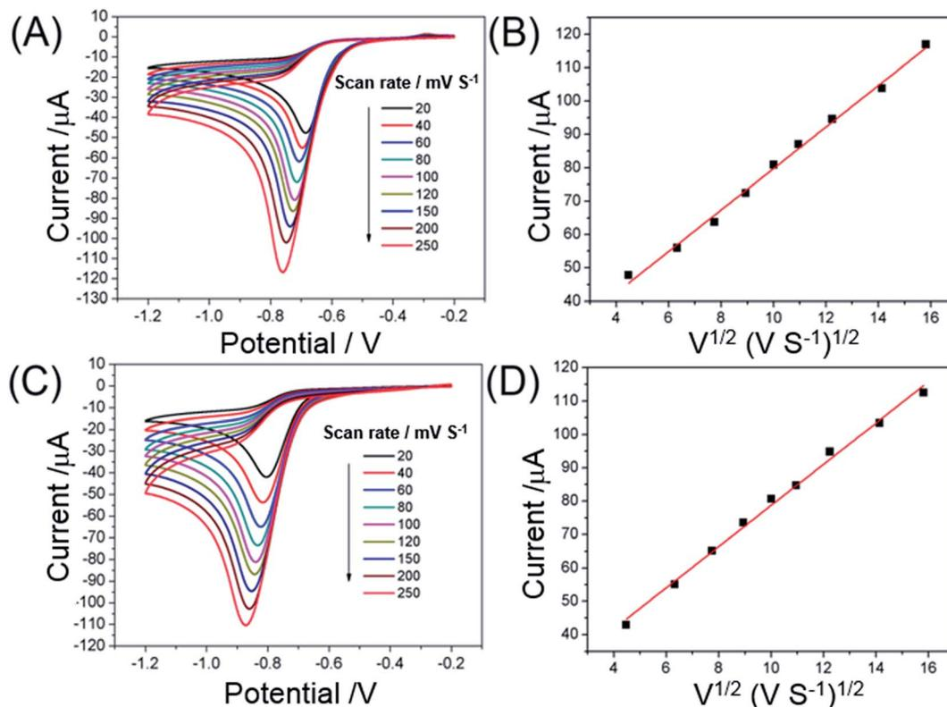
Fig. 4 CVs obtained of the reduction of 1 mM *o*-NP (A, B) and *p*-NP (C, D) at Au-CSiC-SH/NH<sub>2</sub>CD/GCE in 0.1 M PBS (pH 6.0) at various scan rates 20, 40, 60, 80, 100, 120, 150, 200, and 250 mV s<sup>-1</sup>; magnitude of reduction peak current vs. square root of scan rate.
