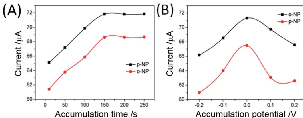
Fig. 3 Effect of accumulation time (A) and accumulation potential (B) on the reduction peak current of 1 mM *o*-NP and *p*-NP at Au-CSiC-SH/NH<sub>2</sub>CD/GCE in 0.1 M PBS (pH 6.0) by DPV. Pulse width: 0.05 s; amplitude: 0.05 V.
