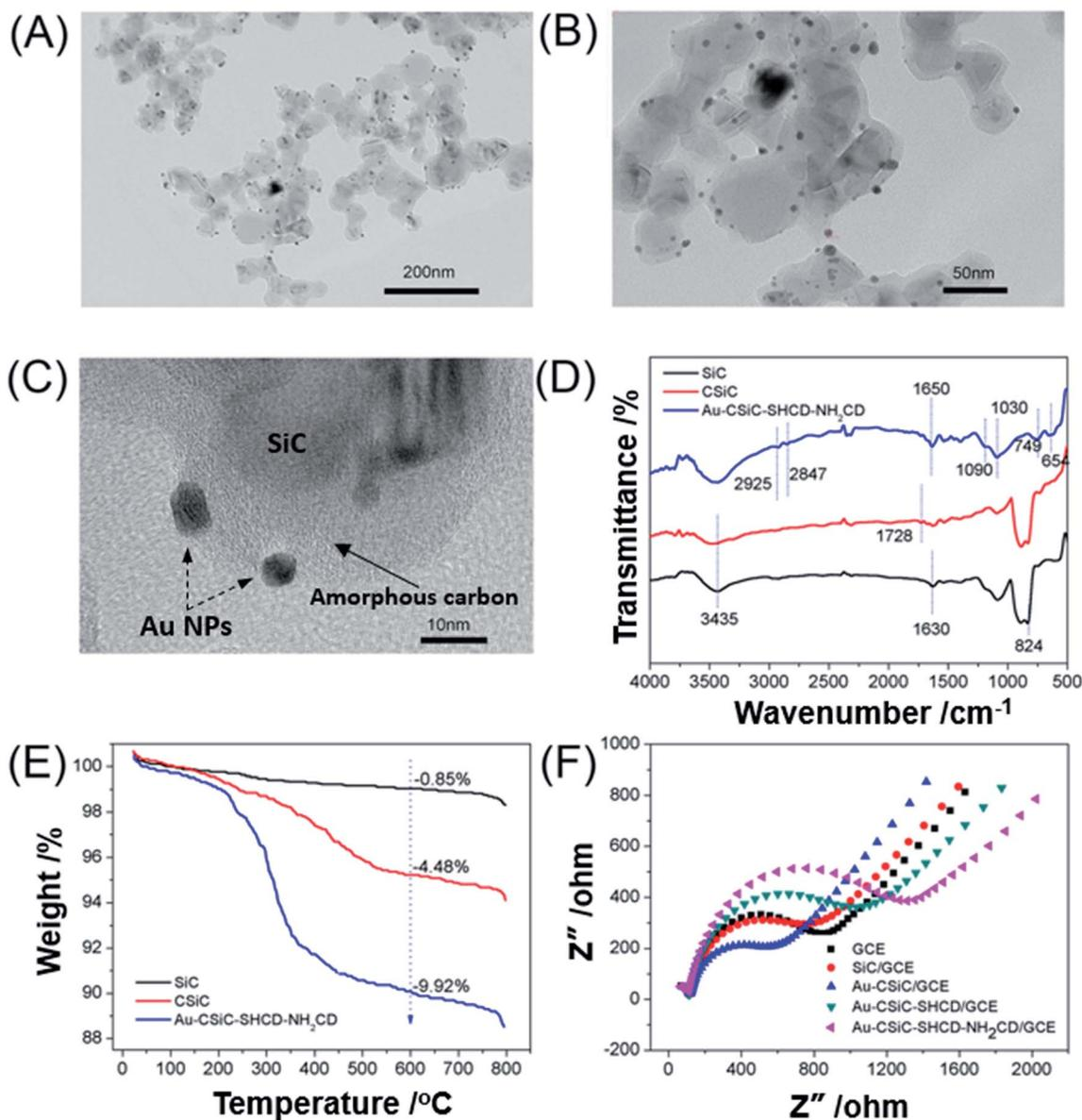
Fig. 1 Characterization of the Au@CSiC and Au@CSiC-SH/NH<sub>2</sub>-CD materials. (A, B, C) TEM images of Au@CSiC at different magnifications; (D) FTIR spectra of SiC, CSiC, and Au@CSiC-SH/NH<sub>2</sub>-CD; (E) TGA curves of SiC, CSiC, and Au@CSiC-SH/NH<sub>2</sub>-CD; (F) EIS characterization of bare GCE, SiC/GCE, Au-SiC/GCE/GCE, Au-SiC-SHCD/GCE, and Au-SiC-SH/NH<sub>2</sub>-CD/GCE using 2.0 mM [Fe(CN)<sub>6</sub>]<sup>3-/4-</sup> redox couple (1 : 1) with 0.1 M KCl as supporting electrolyte.
