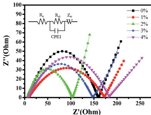
Fig. 9 Impedance spectra of the LNCMA-X% at open circuit voltage. Inset: equivalent circuit corresponding to the impedance diagrams.
