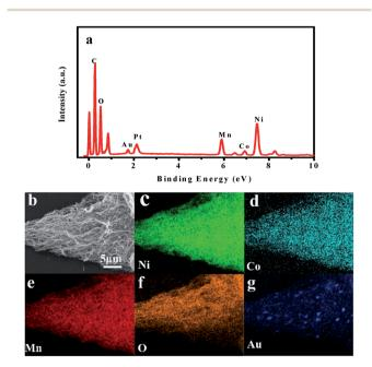
Fig. 4 (a) EDS spectrum, (b) SEM image, and (c-g) EDS elemental mappings of LNCMA-2%.
