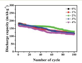
Fig. 7 The cycle capabilities of the LNCMA-X% at 0.2C in the voltage range of 2.0–4.8 V.
