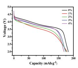
Fig. 6 The initial discharge profiles of the LNCMA-X% at 0.2C in the voltage of 2.0–4.8 V.
