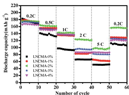
Fig. 8 Rate performance of as-prepared LNCMA- $x\%$  ( $x = 0, 1, 2, 3, 4$ ).
