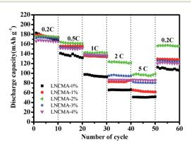
Fig. 8 Rate performance of as-prepared LNCMA-x% (x = 0, 1, 2, 3, 4).
