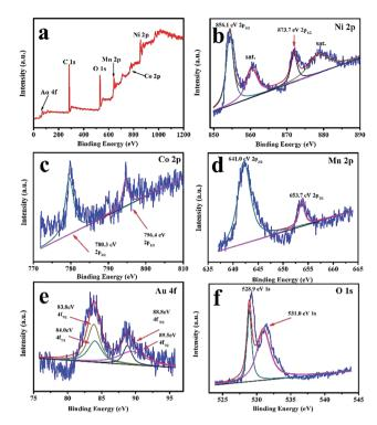
Fig. 5 XPS spectra and corresponding fitting curves of LNCMA-2% nanofibers. (a) Survey spectrum, (b) Ni 2p, (c) Co 2p, (d) Mn 2p, (e) Au 4f, (f) O 1s.
