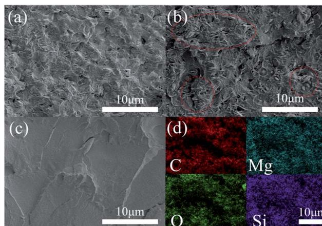
Fig. 5 Freeze-fractured cross-sections of (a) 40 wt% SiO<sub>2</sub>@MgO-PMMA, (b) 40 wt% MgO-PMMA and (c) PMMA films. (d) Element distribution of (a).
