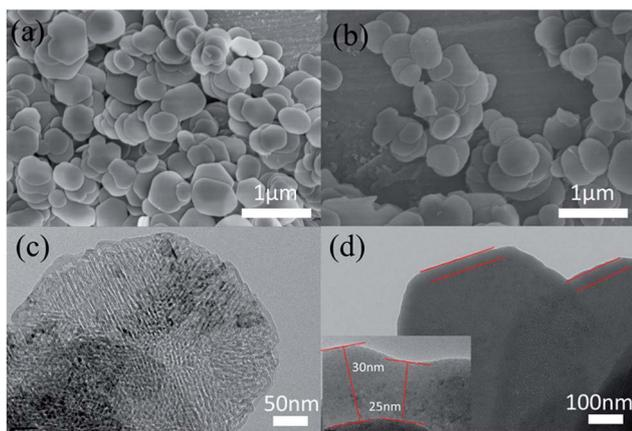
Fig. 3 (a and b) SEM and (c) TEM images of MgO nanosheets; (d) TEM images of core-shell structure of SiO<sub>2</sub>@MgO.
