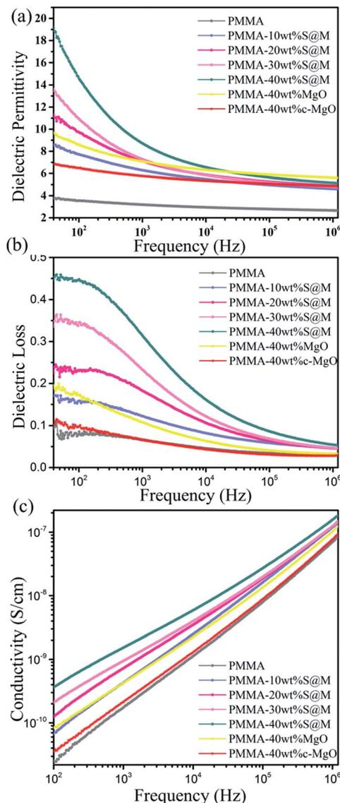
Fig. 8 Frequency dependence of (a) dielectric constant, (b) dielectric loss and (c) conductivity of PMMA, MgO-PMMA and SiO<sub>2</sub>@MgO-PMMA composites with different weight ratios.
