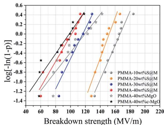
Fig. 9 Weibull plots of the breakdown strength for MgO–PMMA and SiO<sub>2</sub>@MgO–PMMA composites.
