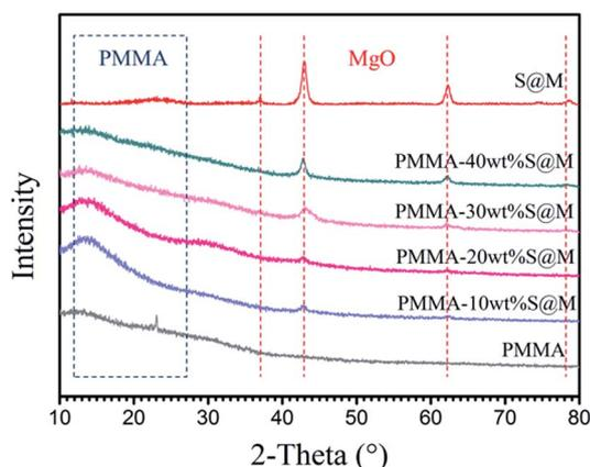
Fig. 4 XRD patterns of SiO<sub>2</sub>@MgO particles, pure PMMA and SiO<sub>2</sub>@MgO-PMMA composites with different weight fractions of SiO<sub>2</sub>@MgO.
