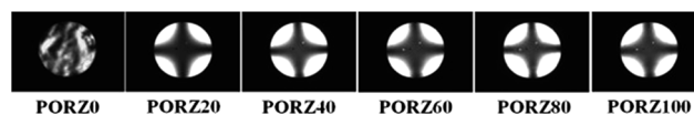
Fig. 6 Conoscopic polarized optical microscopy (POM) images of the LC cells made from PORZ0 (or PCMS) and PORZ20, PORZ40, PORZ60, PORZ80, and PORZ100 films.
