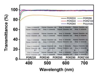
Fig. 3 Optical transmittance spectra of PORZ# and polyimide orientation layers onto quartz substrates.
