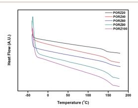
Fig. 2 DSC thermogram of oryzanol modified polystyrene (PORZ#).
