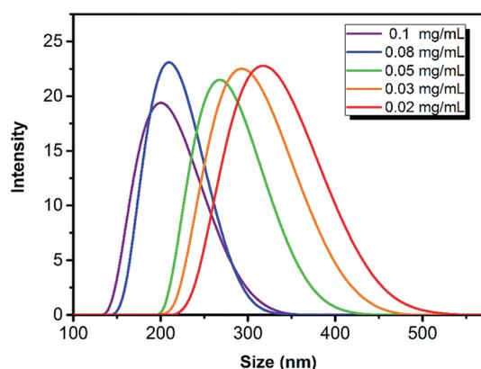
Fig. 2 DLS distributions of NHC with different sizes while the concentration of SDS used is from 0.1 mg mL<sup>-1</sup> (purple) to 0.02 mg mL<sup>-1</sup> (red).
