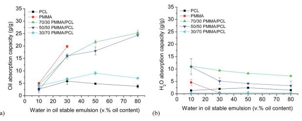
Fig. 3 Simultaneous oil (a) and water (b) absorption capacity of PCL, PMMA, and PMMA/PCL fiber mats in emulsions with oil contents from 10 to 80 v%.
