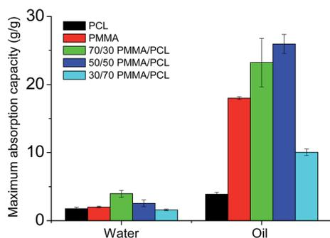
Fig. 2 Maximum water and oil absorption capacity of the fibers after 15 min of full immersion in the respective liquids.
