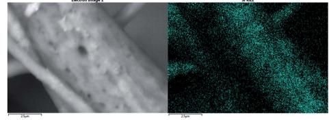
Fig. 4 (a) SEM micrographs and diameter distribution (inset) of SNP/PMMA/PCL fibers with 1.0 wt% SNPs, and (b) SEM image with higher magnification and the corresponding EDS map showing a homogeneous distribution of Si (green color) on the surface of the fibers.
