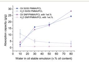
Fig. 5 Simultaneous oil and water absorption capacity of 50/50 PMMA/PCL and SNP/PMMA/PCL fiber mats in emulsions with oil contents from 10 to 80  $\nu$ %.
