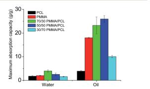
Fig. 2 Maximum water and oil absorption capacity of the fibers after 15 min of full immersion in the respective liquids
