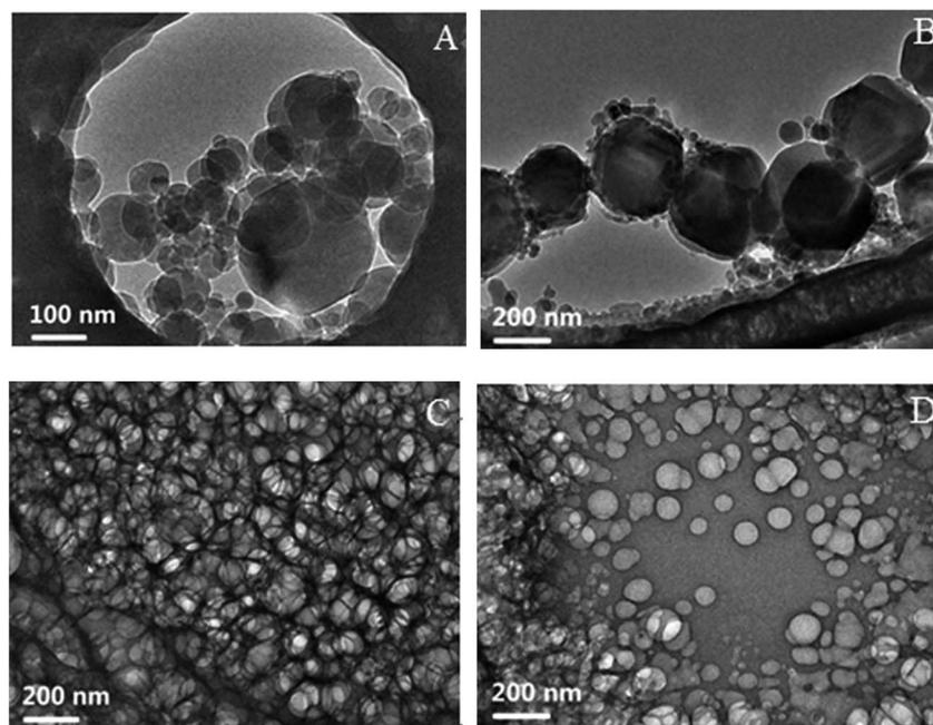
Fig. 5 Cryo-TEM images of the samples (A) *a*, (B) *b*, (C) *c*, and (D) *d*. The samples *a* and *b* fall in the O/W subregion, and the samples *c* and *d* fall in the BC and W/O subregions, respectively, as marked in Fig. 1.
