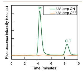
Fig. 3 Isocratic separation of two NNIs and PIF detection at  $\lambda_{ex}/\lambda_{em} =$ 332/368 nm for IMI and  $\lambda_{ex}/\lambda_{em}=353/408$  nm for CLT, respectively.
