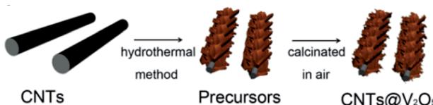
Fig. 13 Schematic of the synthesis process for CNTs@ $\text{V}_2\text{O}_5$ .<sup>127</sup>
