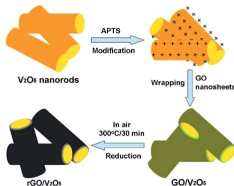
Fig. 14 Schematic of the fabrication of rGO enwrapped  $\text{V}_2\text{O}_5$  nanorods.<sup>140</sup>
