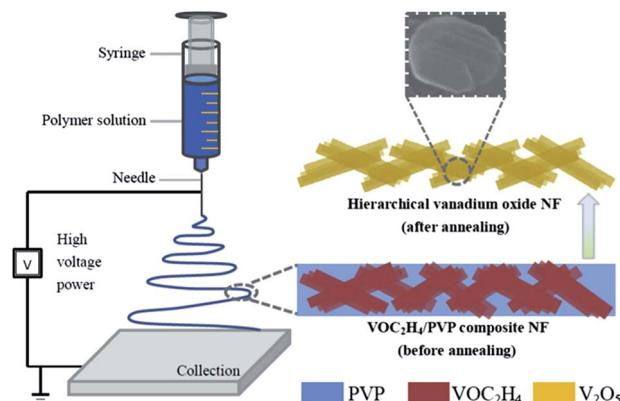
Fig. 6 Schematic showing the strategy for fabricating hierarchical  $\text{V}_2\text{O}_5$  nanofibers.<sup>79</sup>
