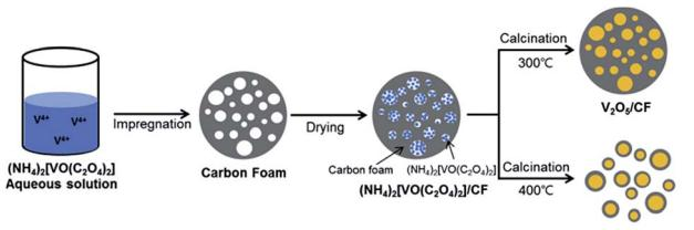
Fig. 12 Schematic of the preparation of carbon-fabricated  $V_2O_5$  samples (CF300 and CF400).<sup>117</sup>
