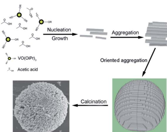
Fig. 11 Schematic of the formation of 3D porous  $V_2O_5$  hierarchical microspheres.<sup>103</sup>
