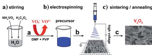
Fig. 3 Electrosynthesis reaction process for  $\text{V}_2\text{O}_5$  micro/nanorods.<sup>54</sup>
