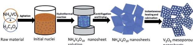
Fig. 9 Schematic of the synthesis route of V<sub>2</sub>O<sub>5</sub> mesoporous nanosheets in this work.<sup>89</sup>
