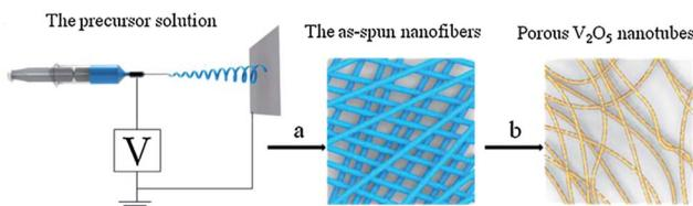
Fig. 5 Electrospinning preparation of porous  $\text{V}_2\text{O}_5$  nanotubes: (a) electrospinning process; (b) annealing process.<sup>76</sup>
