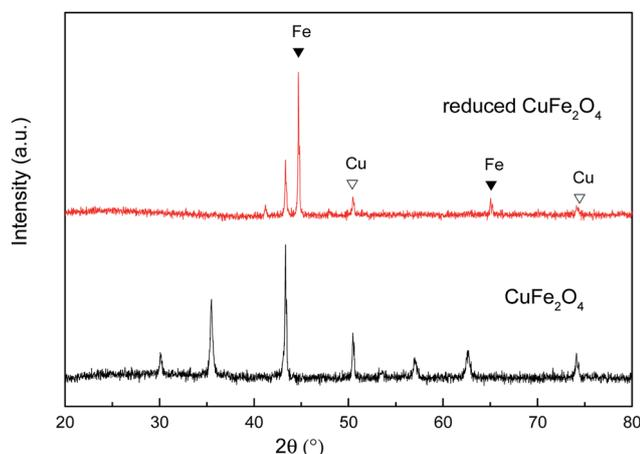
Fig. 2 XRD patterns of  $\text{CuFe}_2\text{O}_4$  and reduced  $\text{CuFe}_2\text{O}_4$ .
