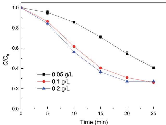
Fig. 6 Effect of catalyst dose on MB degradation by reduced  $\text{CuFe}_2\text{O}_4$ . Conditions:  $[\text{H}_2\text{O}_2] = 0.5 \text{ mM}$ ,  $[\text{MB}] = 50 \text{ mg L}^{-1}$ , initial  $\text{pH} = 3.2 \pm 0.1$ .
