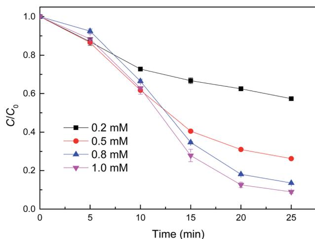
Fig. 7 Effect of  $\text{H}_2\text{O}_2$  concentration on MB degradation by reduced  $\text{CuFe}_2\text{O}_4$ . Conditions:  $[\text{reduced CuFe}_2\text{O}_4] = 0.1 \text{ g L}^{-1}$ ,  $[\text{MB}] = 50 \text{ mg L}^{-1}$ , initial  $\text{pH} = 3.2 \pm 0.1$ .
