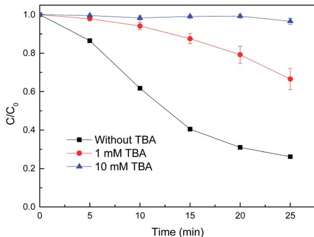
Fig. 10 Effect of TBA on MB degradation by reduced  $\text{CuFe}_2\text{O}_4$ . Conditions:  $[\text{H}_2\text{O}_2] = 0.5 \text{ mM}$ ,  $[\text{reduced CuFe}_2\text{O}_4] = 0.1 \text{ g L}^{-1}$ ,  $[\text{MB}] = 50 \text{ mg L}^{-1}$ , initial  $\text{pH} = 3.2 \pm 0.1$ .
