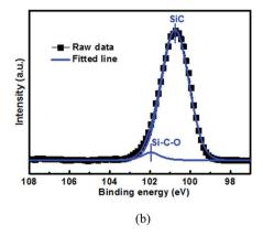
Fig. 1 Si 2p XPS spectrum for the 500 nm (a) Si anode film and (b) SiC anode film before electrochemical cycling. The samples are sputtered by Ar+ for 1 min before test.
