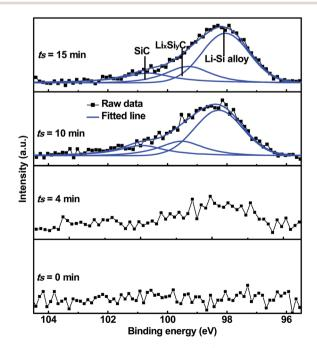
Fig. 5 Si 2p XPS spectrum as a function of Ar<sup>+</sup> sputtering time for the 500 nm SiC anode film at a fully discharge (0.01 V) state.
