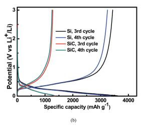
Fig. 4 Charge/discharge voltage profiles for the 500 nm Si and SiC and samples at a current density of 0.01C (a) in the 1st cycle; (b) in the 3<sup>rd</sup> and 4<sup>th</sup> cycles. The inset of Fig. 3(a) shows that the SiC sample displays a slope in the range of 0.5-1.5 V followed by a voltage overshoot at the initial stage of the 1st discharge process.
