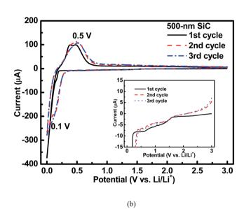
Fig. 3  $\,$  CV profiles of the 500 nm (a) Si sample and (b) SiC sample. The inset shows that there is an extra cathodic peak between 0.5–1.5 V for the SiC sample compared with the Si one.
