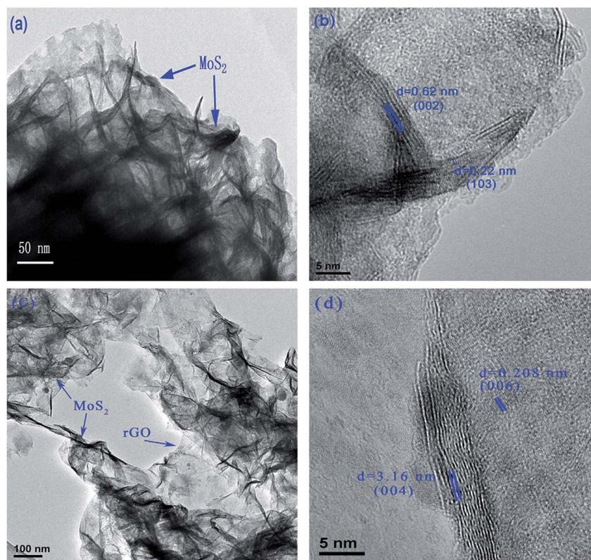
Fig. 3 Typical HRTEM images of MoS<sub>2</sub> (a and b) and MoS<sub>2</sub>/rGO (1 : 2) (c and d) composite.
