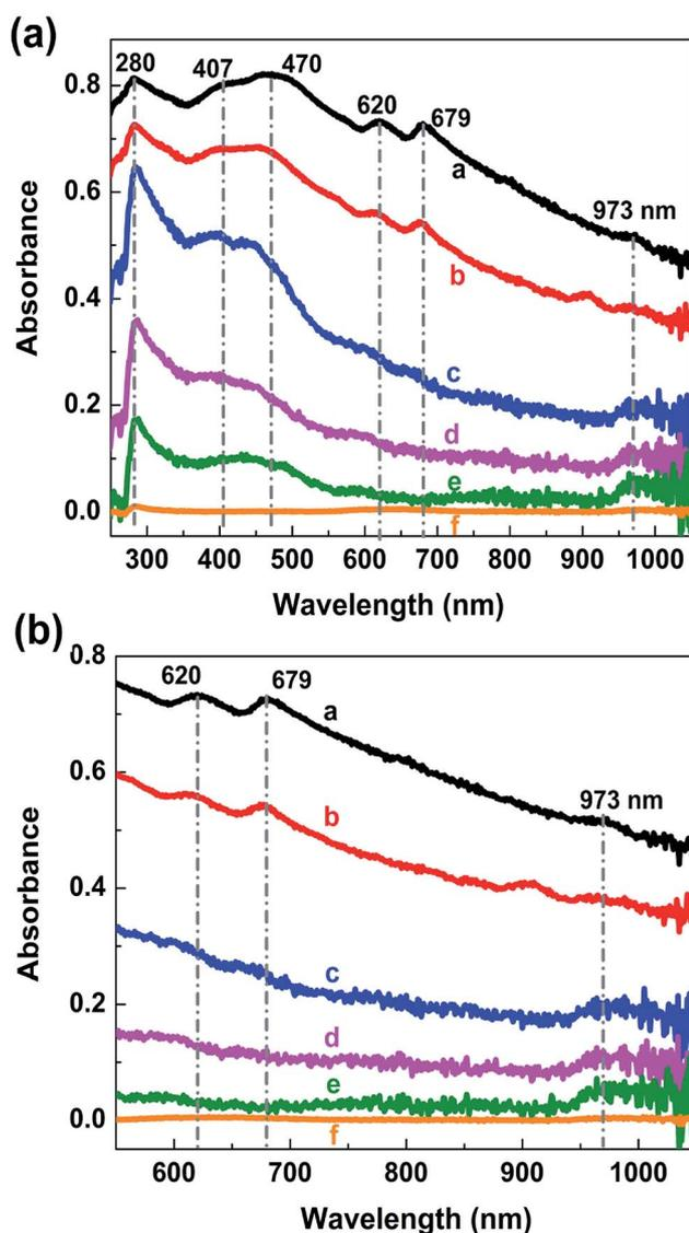
Fig. 6 The absorption spectra of MoS<sub>2</sub>/rGO composites from ultraviolet to infrared region (a) and from red to infrared region (b), obtained at different centrifugation speeds: a-3500 rpm, b-5000 rpm, c-6500 rpm, d-8000 rpm, e-9500 rpm, f-11 000 rpm.
