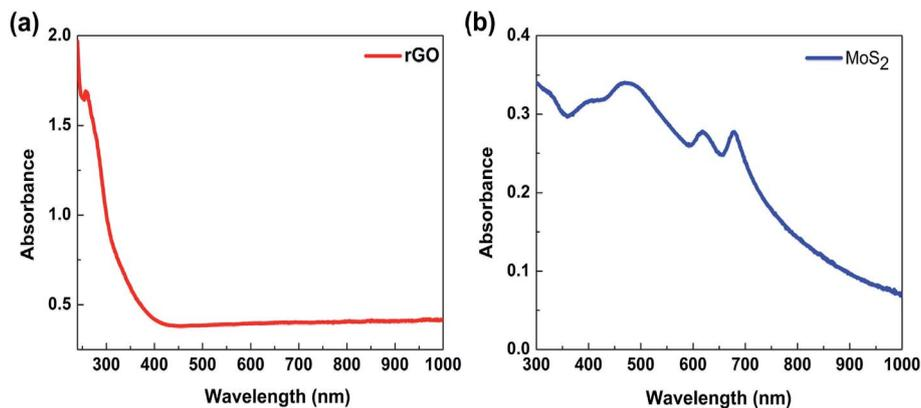
Fig. 5 Absorption spectra of rGO (a) and few layer MoS<sub>2</sub> nanosheets (b).
