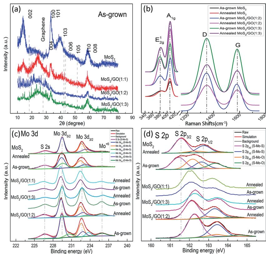
Fig. 2 XRD patterns (a), Raman (b) and XPS (c, d) spectra of MoS<sub>2</sub>/rGO with different MoS<sub>2</sub>/GO ratios for Mo 3d (c) and S 2p (d).
