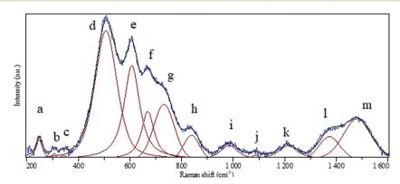
Fig. 4 Raman spectrum of BaCO<sub>3</sub>/BaSnO<sub>3</sub>/SnO<sub>3</sub> nanocomposite.
