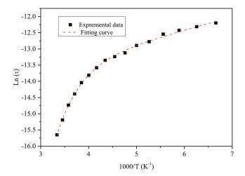
Fig. 10 Temperature dependence of the  $tan(\delta)$  relaxation time of the nanocomposite. Symbol (black) represents experimental data. The dashed line (red) corresponds to the best fit according to the eqn (5).
