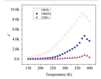
Fig. 7 Temperature dependence of the dielectric constant measured at different frequencies.
