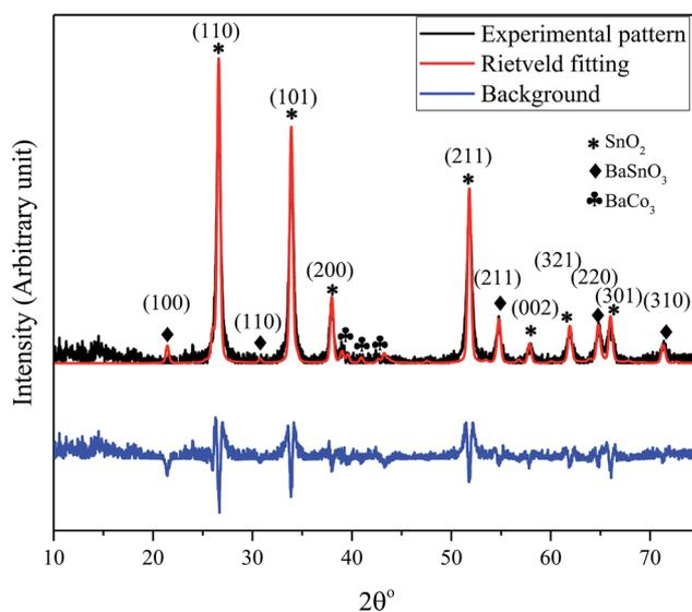
Fig. 1 XRD pattern and the Rietveld refinement of BaCO<sub>3</sub>/BaSnO<sub>3</sub>/SnO<sub>2</sub> nanocomposite powder along with the crystal plan indexation for the main phases.
