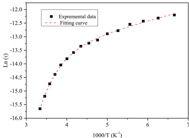
Fig. 10 Temperature dependence of the  $\tan(\delta)$  relaxation time of the nanocomposite. Symbol (black) represents experimental data. The dashed line (red) corresponds to the best fit according to the eqn (5).
