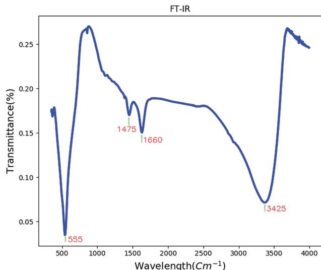
Fig. 3 The FT-IR spectrum of BaCO<sub>3</sub>/BaSnO<sub>3</sub>/SnO<sub>2</sub> nanocomposite.
