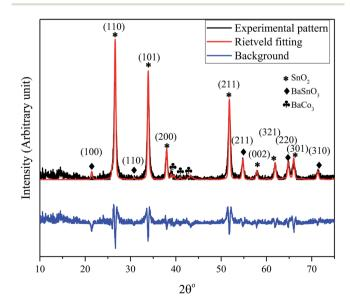
Fig. 1 XRD pattern and the Rietveld refinement of  $BaCO_3/BaSnO_3/SnO_2$  nanocomposite powder along with the crystal plan indexation for the main phases.
