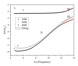
Fig. 8 Variation of ac conductivity ( $\sigma_{ac}$ ) as function of frequency at different temperatures (K): (a) 280, 300 and 320; (b): 340, 360 and 400.
