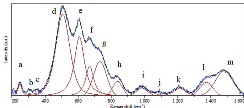
Fig. 4 Raman spectrum of BaCO<sub>3</sub>/BaSnO<sub>3</sub>/SnO<sub>3</sub> nanocomposite.
