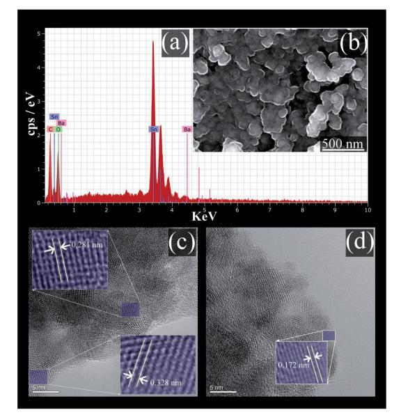
Fig. 2 (a) The EDS spectrum; (b) SEM micrograph; (c) and (d) HRTEM images of BaCO<sub>3</sub>/BaSnO<sub>3</sub>/SnO<sub>2</sub> nanocomposite
