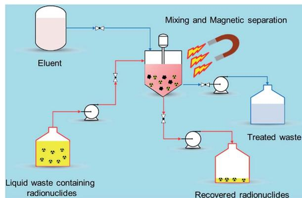
Fig. 2 Magnetic assisted separation for radionuclides from wastewater.
