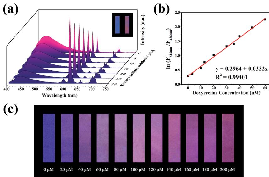
Fig. 3 (a) Fluorescence spectra of composites with different concentrations of doxycycline under 298 nm excitation. (b) The linear relationship of  $\ln(F_{616\text{ nm}}/F_{436\text{ nm}})$  and concentration of doxycycline. (c) The colour change of "test paper" as the concentration of doxycycline increased under 365 nm UV irradiation.
