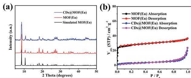
Fig. 2 (a) Comparison of the XRD patterns of MOF(Eu) and CDs@MOF(Eu) composite. (b) N<sub>2</sub> absorption–desorption isotherms of MOF(Eu) and CDs@MOF(Eu).
