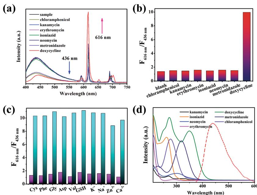
Fig. 4 (a) Fluorescence spectra of composites added with different antibiotics. (b) Selectivity of doxycycline based on the ratio of  $F_{616\text{ nm}}$  and  $F_{436\text{ nm}}$ . (c) Value of  $F_{616\text{ nm}}/F_{436\text{ nm}}$  in the presence of other interfering substances (excited at 298 nm). (d) Absorption spectrum of different antibiotics and emission spectra of carbon dots.
