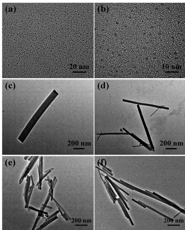
Fig. 1 Transmission electron micrographs of carbon dots (a and b), CDs@MOF(Eu) (c and d) and MOF(Eu) (e and f).
