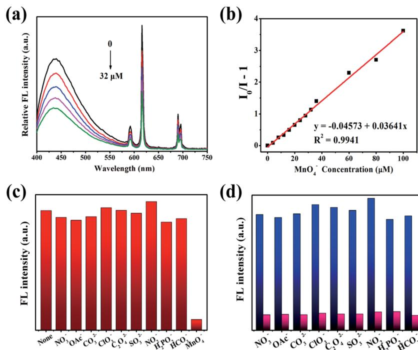
Fig. 5 (a) Emission spectra of CDs@MOF(Eu) with added MnO<sub>4</sub><sup>-</sup> (0–32 μM). (b) The linear relationship between MnO<sub>4</sub><sup>-</sup> concentration and I<sub>0</sub>/I - 1 based on the 616 nm emission peak. (c) The selectivity of MnO<sub>4</sub><sup>-</sup> with that of other anions. (d) Fluorescence intensity at 616 nm of composites with added MnO<sub>4</sub><sup>-</sup> (0.2 mM) in the interference of other anions (0.2 mM).
