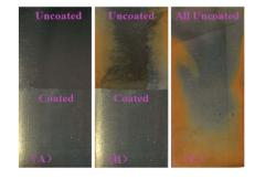
Fig. 5 Image of tin plate coated or uncoated after immersion in NaCl solution.
