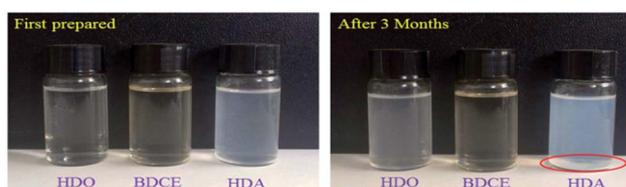
Fig. 9 Storage stability of different polyurethane coatings.
