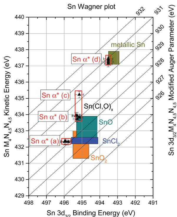
Fig. 7 Sn modified Auger parameter ( $\alpha^*$ ) of the investigated sample series in a Wagner plot format. Illustrated as shaded area are BE and KE values of reference Sn compounds reported in literature.<sup>30–36</sup>
