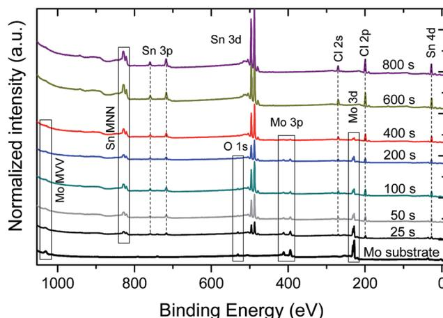
Fig. 1 Mg  $K_{\alpha}$ -excited XPS survey spectra of the  $\text{SnCl}_2$  thin-film thickness series on Mo, along with identification of core level and Auger lines. Vertical offsets are added for clarity.
