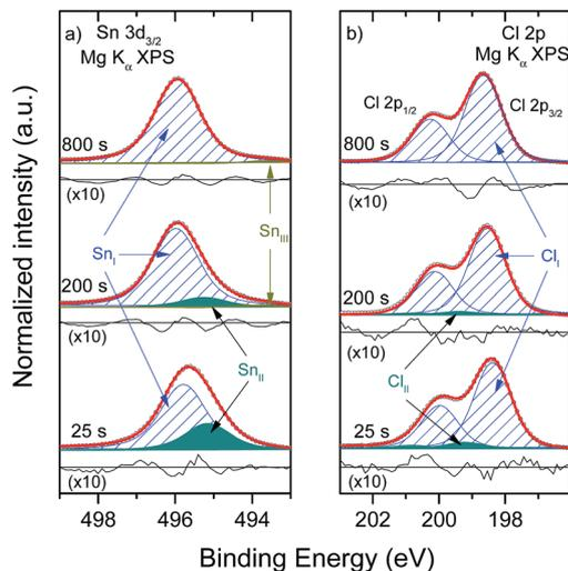
Fig. 5 XPS detail spectra of the (a) Sn  $3d_{3/2}$  and (b) Cl 2p energy regions of the “25 s”, “200 s” and “800 s” samples, including fits and respective residua. Spectra are normalized to maximum intensity.
