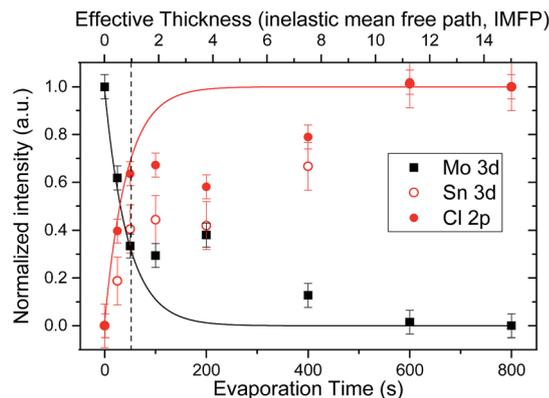
**Fig. 3** Relative intensities of Sn 3d, Cl 2p, and Mo 3d lines as a function of SnCl<sub>2</sub> evaporation time in the sample series. The solid lines show intensity evolutions expected of a homogeneous layer-by-layer deposition of SnCl<sub>2</sub> as a function of its effective thickness (in multiples of IMFP values). The vertical dashed line indicates a SnCl<sub>2</sub> effective thickness equal to one IMFP value (*i.e.*, *ca.* 2 nm).<sup>†</sup>
