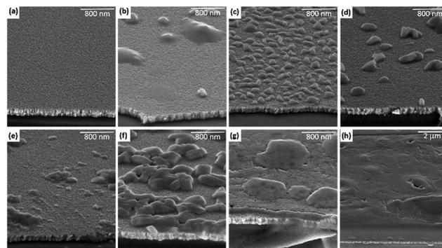
Fig. 2 30°-Tilted cross section scanning electron microscope (SEM) images of  $\text{SnCl}_2/\text{Mo}$  samples with the following evaporation times: (a) 25 s, (b) 50 s, (c) 100 s, (d) 200 s, (e) 400 s, (f) 600 s, (g) 800 s, and (h) 1600 s. SEM images (a)–(g) were taken with a 30 000 $\times$  magnification, whereas (h) shows a 10 000 $\times$  magnification.
