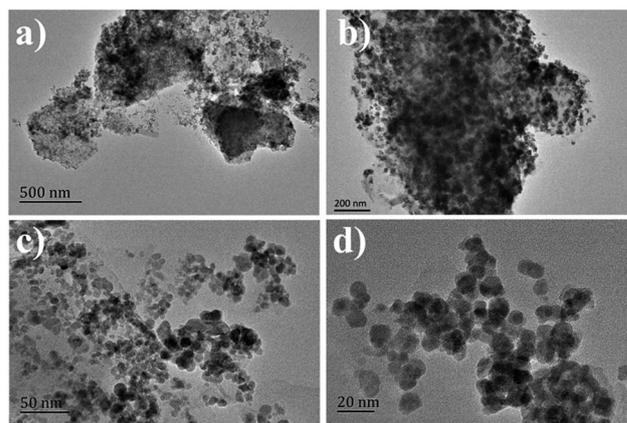
Fig. 2 TEM of the  $\text{CeMo}_{0.15}\text{O}_x\text{-OC-550}$  catalyst.
