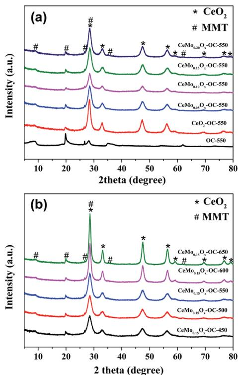
Fig. 1 XRD patterns of (a)  $\text{CeMo}_x\text{O}_y\text{-OC-550}$  catalysts with different Mo/Ce ratios, (b)  $\text{CeMo}_{0.15}\text{O}_x\text{-OC-}T$  catalysts with different calcination temperature.
