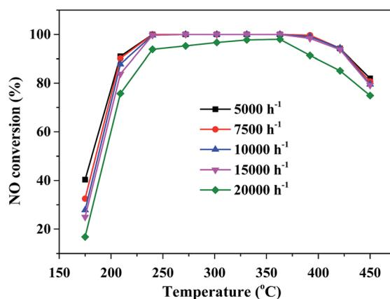
Fig. 7 NO<sub>x</sub> conversion of CeMo<sub>0.15</sub>O<sub>x</sub>-OC-550 catalyst in the difference space velocity.
