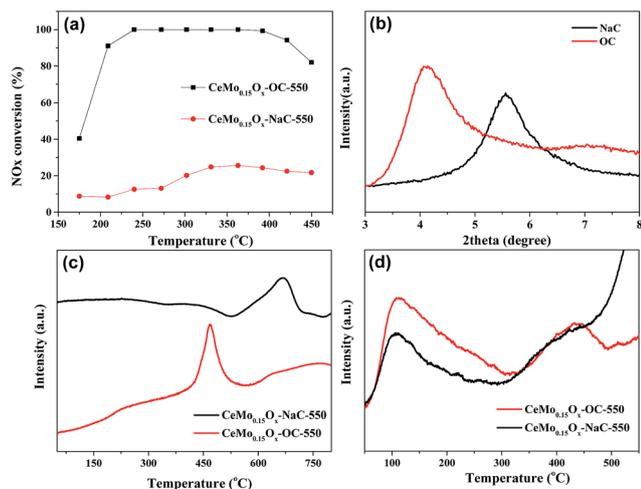
Fig. 6 The NO<sub>x</sub> conversion (a), XRD (b), H<sub>2</sub>-TPR (c), NH<sub>3</sub>-TPD (d) of CeMo<sub>0.15</sub>O<sub>x</sub>-OC-550 and CeMo<sub>0.15</sub>O<sub>x</sub>-NaC-550 catalysts.
