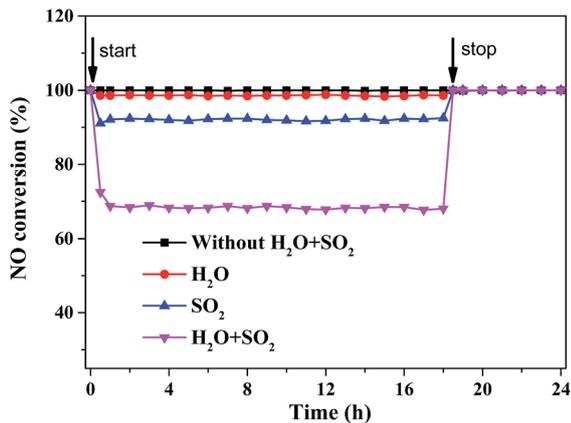
Fig. 8 NO<sub>x</sub> conversion of CeMo<sub>0.15</sub>O<sub>x</sub>-OC-550 catalyst with different conditions in the presence of 5 vol% H<sub>2</sub>O, 200 ppm SO<sub>2</sub> and 5 vol% H<sub>2</sub>O + 200 ppm SO<sub>2</sub>, respectively, at 5000 h<sup>-1</sup>, 330 °C.
