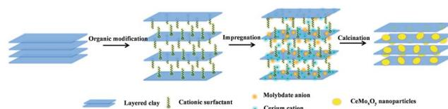
Scheme 1 Illustration for the preparation of CeMo<sub>x</sub>O<sub>y</sub>-OC-*T* catalysts.
