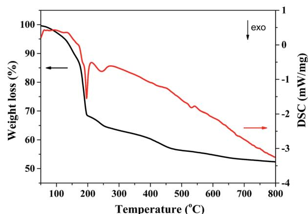
Fig. 3 TG-DSC profiles of the as-prepared  $\text{CeMo}_{0.15}\text{O}_x\text{-OC}$  precursor.
