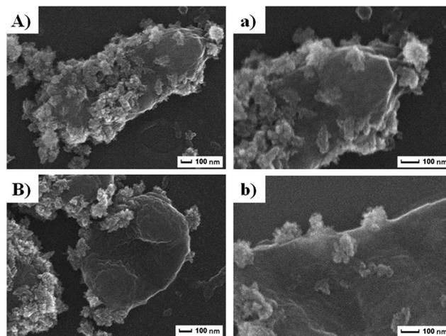
Fig. 5 (A and B) were SEM images of MDR *E. coli* and MRSA after treatment with Zn-CuO@GO, respectively. (a and b) were magnified SEM images revealing detailed cell-material interactions.
