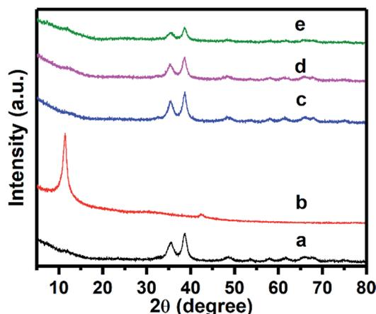
Fig. 2 XRD pattern of Zn–CuO (a), GO (b), Zn–CuO@GO (4 : 1) (c), Zn–CuO@GO (2 : 1) (d), and Zn–CuO@GO (1 : 1) (e), respectively.
