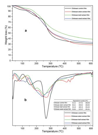
Fig. 2 (a) TGA and (b) DTG thermograms of the chitosan control film and blend films incorporated with *Pistacia terebinthus*' extracts as; chitosan-stem film, chitosan-leaf film and chitosan-seed film.
