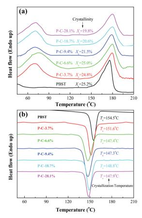
Fig. 4 Heating scan (a) and cooling scan (b) in the DSC curves obtained for the PBST composite nanofibrous membranes.
