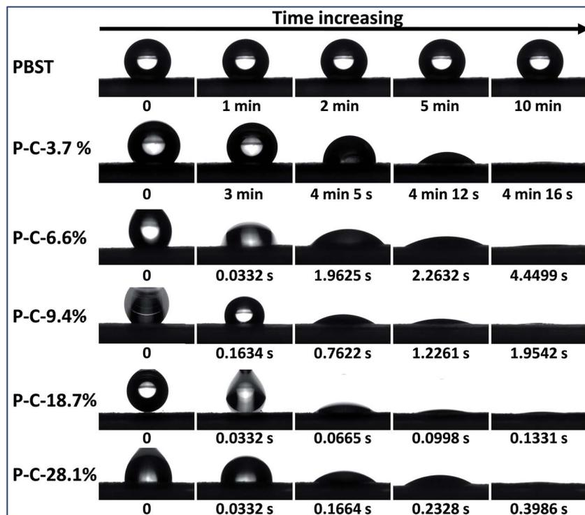
Fig. 6 Evolution of a water droplet placed on the PBST composite nanofibrous membranes with time.
