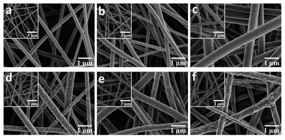
Fig. 2 SEM images of the nanofibrous membranes: (a) pure PBST, (b) P-C-3.7%, (c) P-C-6.6%, (d) P-C-9.4%, (e) P-C-18.7% and (f) P-C-28.1% (the insets are the corresponding images at lower magnification).
