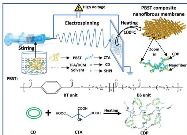
Fig. 1 Schematic representation of the preparation of PBST composite nanofibrous membrane.
