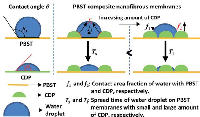
Fig. 7 Illustration showing the evolution of the water contact angle of the PBST composite nanofibrous membranes.
