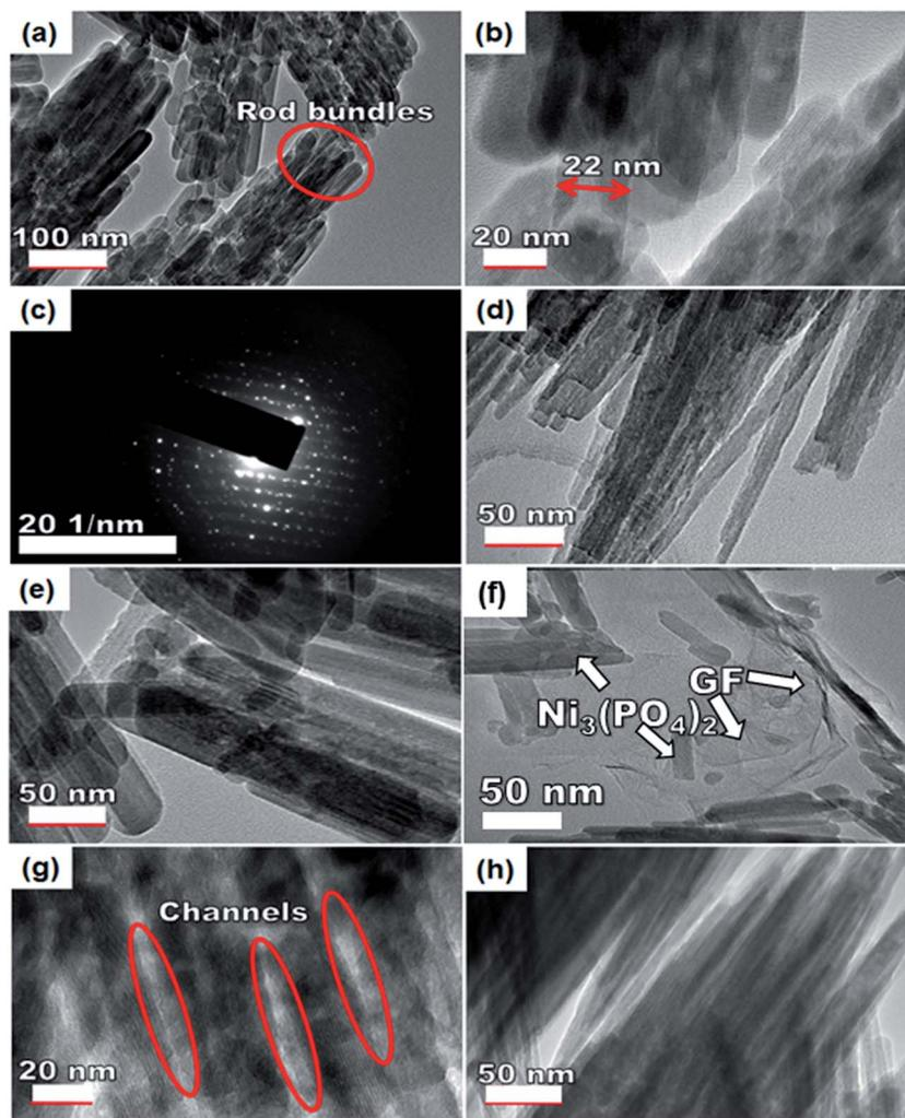
Fig. 4 An HRTEM image of the (a and b) pristine  $\text{Ni}_3(\text{PO}_4)_2$  sample at low and high magnification and the corresponding (c) SAED image of the pristine sample, (d)  $\text{Ni}_3(\text{PO}_4)_2/30$  mg GF, (e)  $\text{Ni}_3(\text{PO}_4)_2/60$  mg GF, (f)  $\text{Ni}_3(\text{PO}_4)_2/90$  mg GF, (g) the channel-like structures of  $\text{Ni}_3(\text{PO}_4)_2/90$  mg GF and (h)  $\text{Ni}_3(\text{PO}_4)_2/120$  mg GF.
