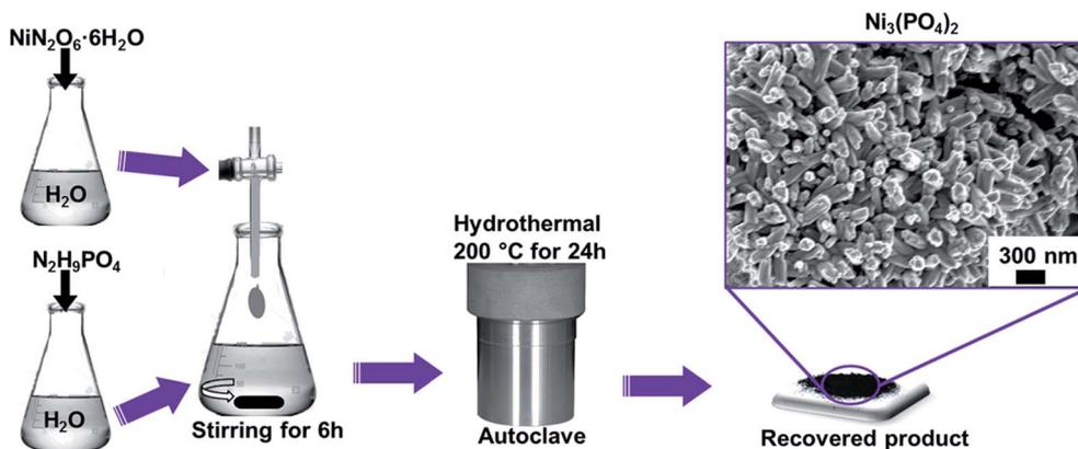
Scheme 1 Preparation procedure of nanostructured nickel phosphate.
