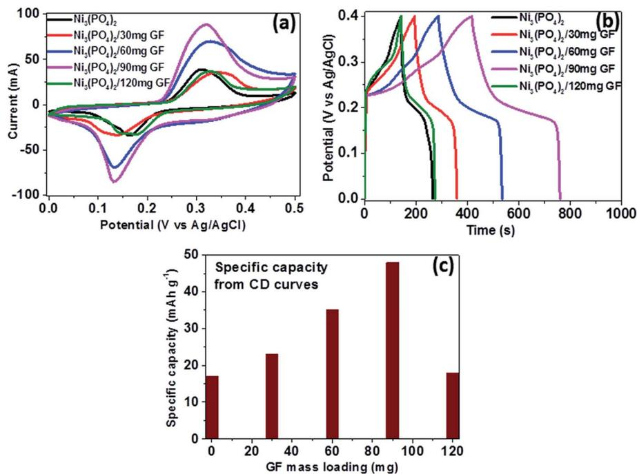
Fig. 5 (a) CV curves of pristine Ni<sub>3</sub>(PO<sub>4</sub>)<sub>2</sub> and Ni<sub>3</sub>(PO<sub>4</sub>)<sub>2</sub>/GF composites at different GF mass loading at a scan rate of 50 mV s<sup>-1</sup>, (b) CD curves of pristine and composites at a current density of 0.5 A g<sup>-1</sup> within a potential window range of 0.0–0.4 V and (c) specific capacity for pristine and composites calculated from the CD curves in (b).
