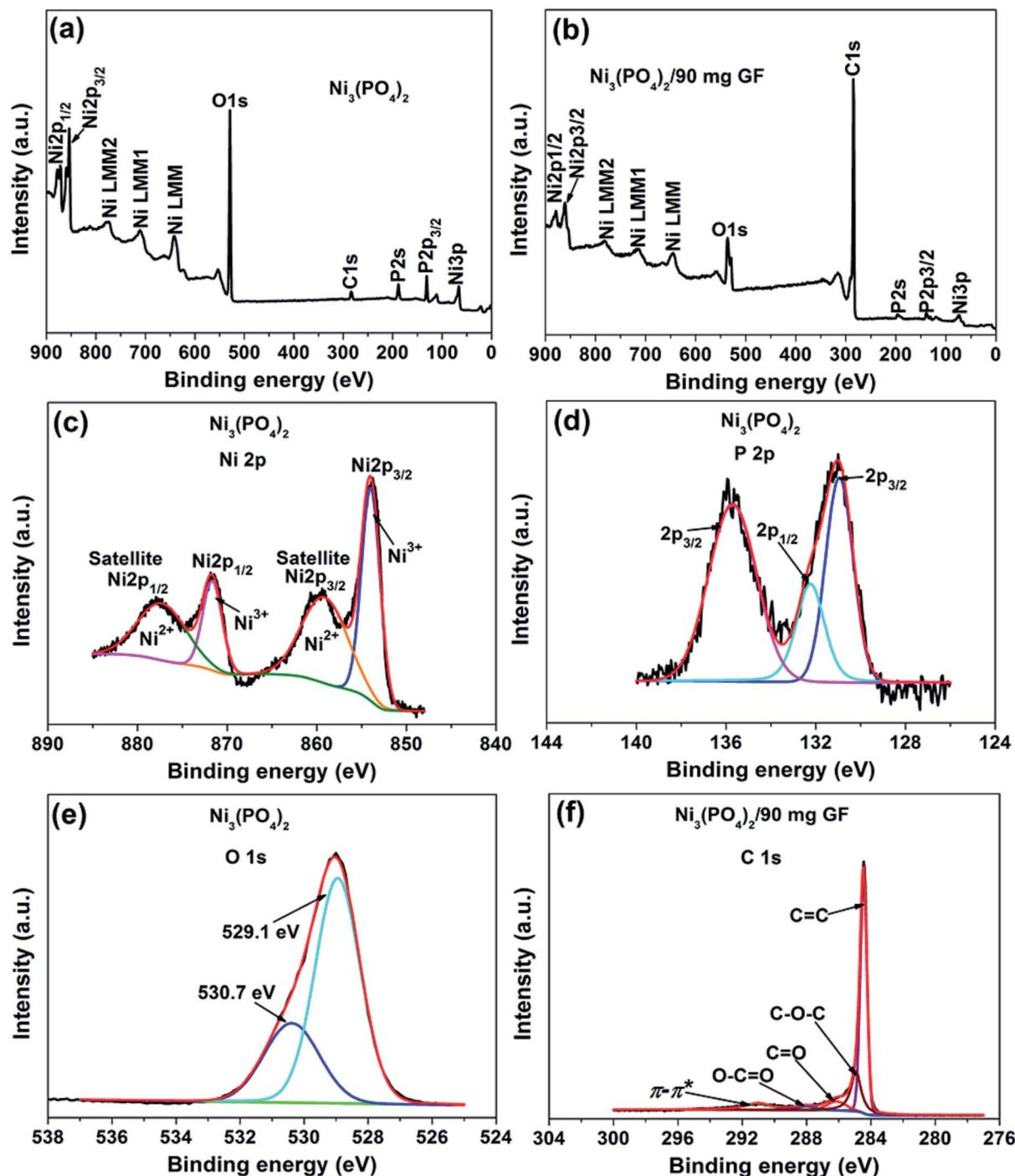
Fig. 2 (a) and (b) The wide scan XPS spectra of the as-received pristine nickel phosphate sample and the  $\text{Ni}_3(\text{PO}_4)_2/90$  mg GF composite respectively. The core level spectrum of (c) Ni 2p, (d) P 2p and (e) O 1s of a pristine sample. (f) The core level spectrum of C 1s of a composite sample.
