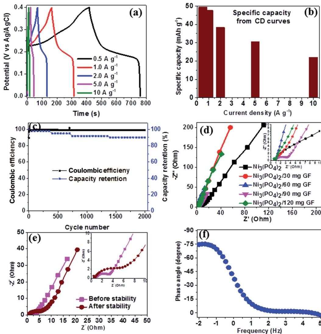
Fig. 6  $\text{Ni}_3(\text{PO}_4)_2/90$  mg GF composite electrochemical data: (a) CD curves at different current densities, (b) specific capacity as a function of current density, (c) the cycling stability at a current density of  $10 \text{ A g}^{-1}$ , (d) Nyquist plots for the samples shown in the (the insert shows the enlarged high-frequency region of the plot), (e) Nyquist before and after stability test and (f) the phase angle as a function of frequency.
