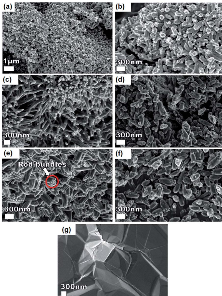
Fig. 3 SEM micrographs of (a and b) pristine  $\text{Ni}_3(\text{PO}_4)_2$  sample at low and high magnification, (c)  $\text{Ni}_3(\text{PO}_4)_2/30$  mg GF, (d)  $\text{Ni}_3(\text{PO}_4)_2/60$  mg GF, (e)  $\text{Ni}_3(\text{PO}_4)_2/90$  mg GF, (f)  $\text{Ni}_3(\text{PO}_4)_2/120$  mg GF and (g) SEM micrograph of a GF sheet before been crushed into powder and sonicated.
