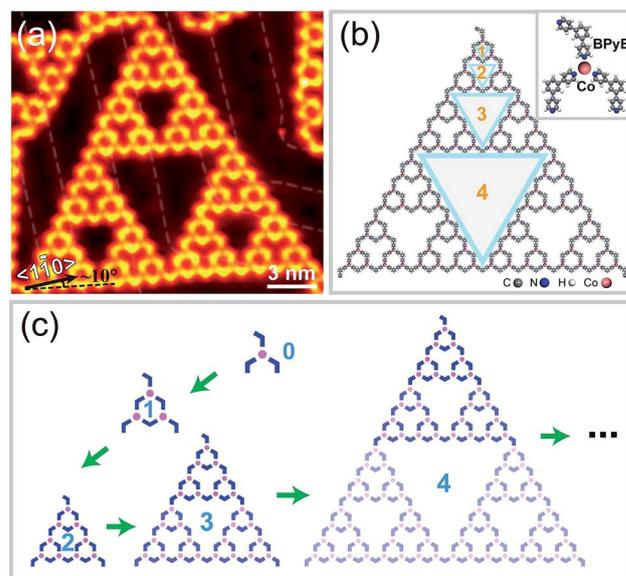
Fig. 1 Fractal phase formed at low molecular coverage. (a) STM image of a defect-free ST of 4 order; inset: coordinated trimer acting as basic recursive unit. The white arrow indicates  $\langle 110 \rangle$  direction. Scanning parameters: constant-height mode,  $V_B = 10$  mV,  $I_t = 80$  pA. (b) Structural model of the ST in (a). (c) Schematic models revealing the evolution process of fractal phase.
