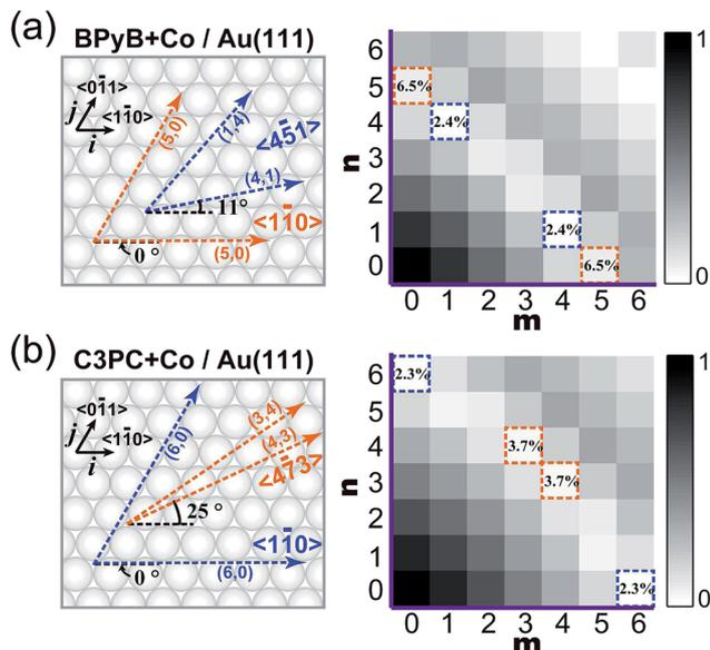
Fig. 5 *K*-Map of (a) BPyB–Co coordination and (b) C3PC–Co coordination. Each left panel corresponds to surface lattice models of Au(111) with the best (blue arrows) and second best (orange arrows) matching orientation; each right panel corresponds to relative gray-scale *K* maps.
