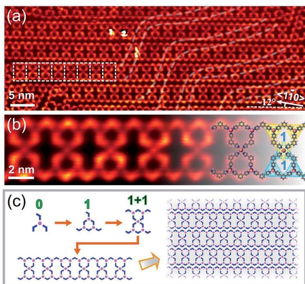
Fig. 3 BPyB-Co-ST-1 arrays formed at high molecular coverage. (a) STM image of 1D molecular ribbons formed by combination of 1 + 1. (b) Detailed STM image of one 1 + 1 ribbon superposed by models. The white arrow points to  $\langle 110 \rangle$  direction. Scanning parameters: constant-height mode, (a)  $V_B = 50$  mV,  $I_t = 60$  pA; (b)  $V_B = 10$  mV,  $I_t = 70$  pA; (c) schematic models indicate the formation of 1D molecular ribbons based on combination 1 + 1.
