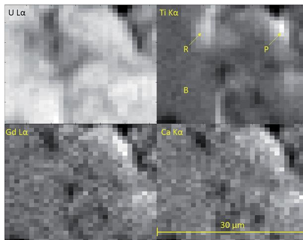
Fig. 6 Fluorescence maps of  $Ca_{0.1}Gd_{0.1}U_{0.72}Ce_{0.08}Ti_2O_6$  sintered in an argon atmosphere. Each pixel represents  $1 \mu m^2$ . Lighter colours indicate higher X-ray fluorescence intensity, darker colours indicate lower intensity. B-brannerite, P-pyrochlore and R-rutile.
