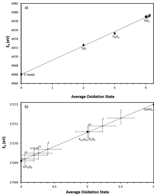
Fig. 5 (a) Linear regression of Ti K edge  $E_0$  values with respect to Ti standards. (b) Linear regression of U L-III edge  $E_0$  values with respect to U standards. Numbers refer to corresponding composition no. in Table 2. Black squares denote standards, open diamonds denote samples.
