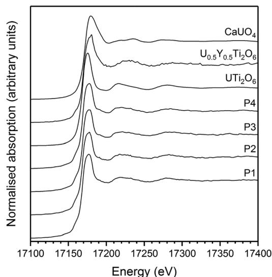
**Fig. 7** Example U L-III edge  $\mu$ -focus XANES for Gd<sub>0.1</sub>U<sub>0.81</sub>Ce<sub>0.09</sub>Ti<sub>2</sub>O<sub>6</sub> synthesised in argon. P1–4 indicate individual spectra taken from separate points.
