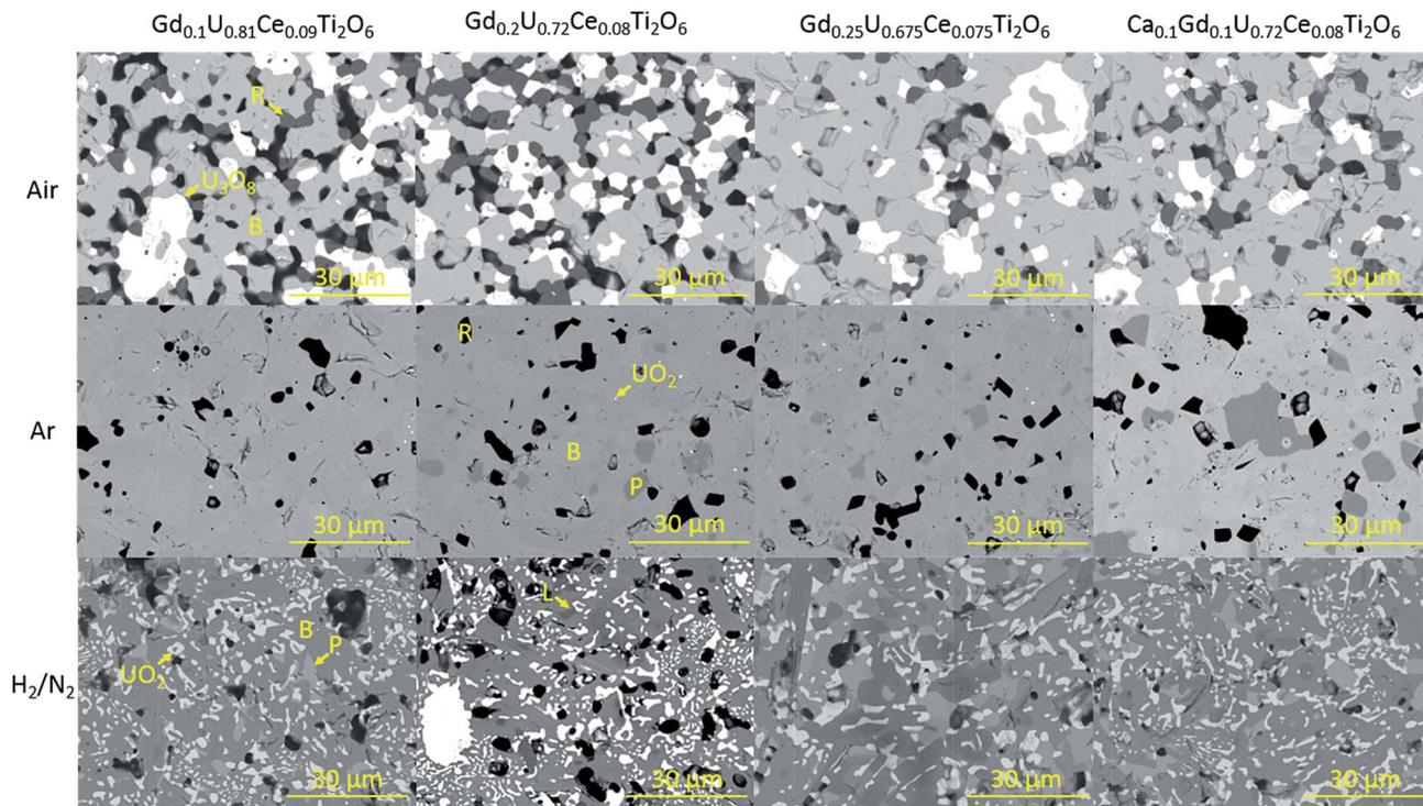
Fig. 2 Representative backscattered electron images of sintered brannerites. B-brannerite, R-rutile, P-pyrochlore, L-Lan<sub>4</sub>Ti<sub>9</sub>O<sub>24</sub>.
