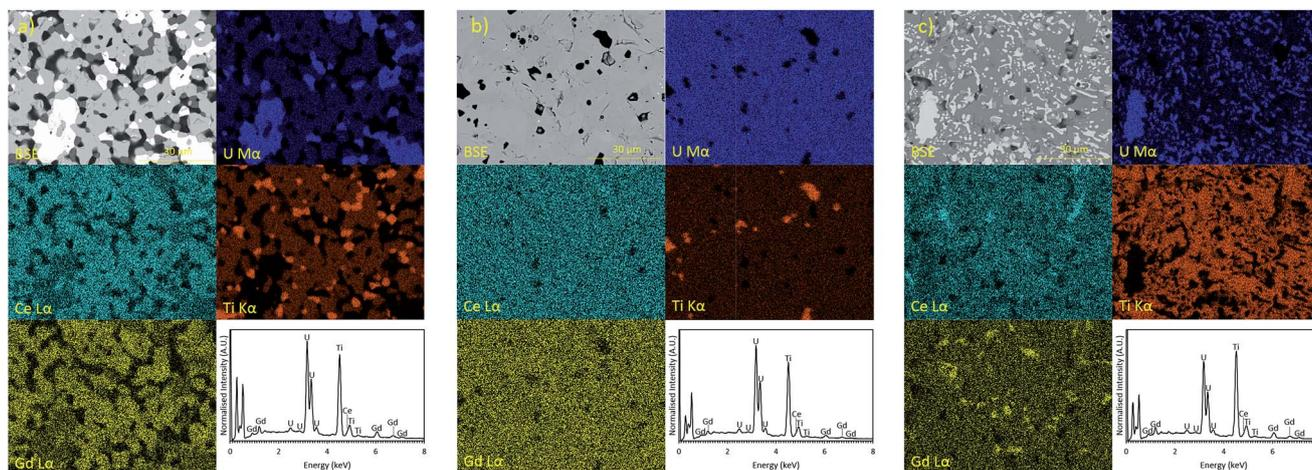
Fig. 3 EDX spectra and elemental partitioning observed in Gd<sub>0.1</sub>U<sub>0.81</sub>Ce<sub>0.09</sub>Ti<sub>2</sub>O<sub>6</sub> synthesised in: (a) air; (b) Argon and (c) 5% H<sub>2</sub>/N<sub>2</sub>.
