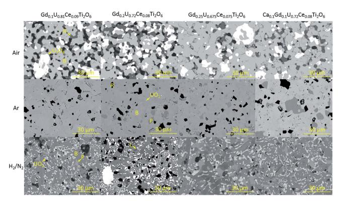
Fig. 2 Representative backscattered electron images of sintered brannerites. B-brannerite, R-rutile, P-pyrochlore, L-Lan<sub>4</sub>Ti<sub>9</sub>O<sub>24</sub>
