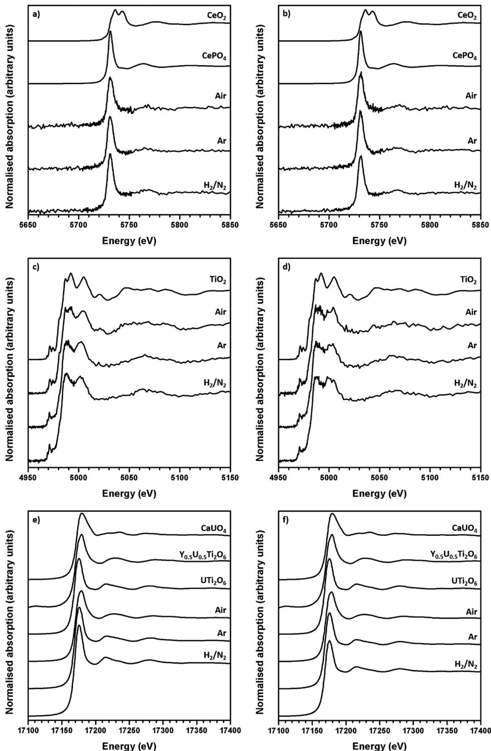
Fig. 4 Representative XANES spectra of synthesised brannerites. (a) Ce  $L_{III}$  edge  $Gd_{0.1}U_{0.81}Ce_{0.1}Ti_2O_6$ ; (b) Ce  $L_{III}$  edge  $Ca_{0.1}Gd_{0.1}U_{0.72}Ce_{0.08}Ti_2O_6$ ; (c) Ti K edge  $Gd_{0.1}U_{0.81}Ce_{0.1}Ti_2O_6$  and (d) Ti K edge  $Ca_{0.1}Gd_{0.1}U_{0.72}Ce_{0.08}Ti_2O_6$ ; (e) U  $L_{III}$  edge  $Gd_{0.1}U_{0.81}Ce_{0.1}Ti_2O_6$  and (f) U  $L_{III}$  edge  $Ca_{0.1}Gd_{0.1}U_{0.72}Ce_{0.08}Ti_2O_6$ .
