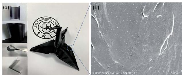
**Fig. 6** (a) Digital photographs of a PEEK/wrapped MWCNT/GPPS1.0 composite film with excellent flexibility, *i.e.*, round into a roll, under bending condition and fold into paper crane shape. (b) Cross-section SEM image of composite film.
