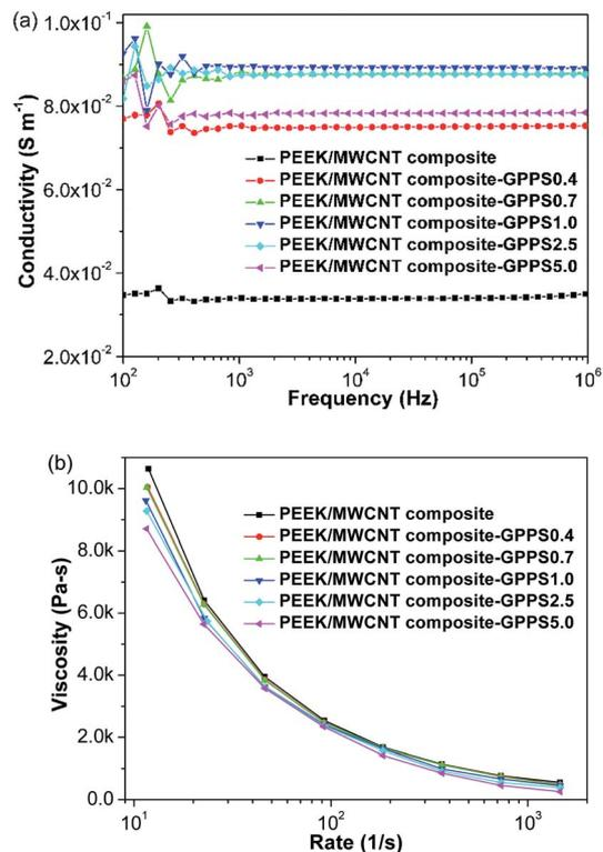
Fig. 1 (a) Dependence of AC conductivity of PEEK/MWCNT composite-GPPS $x$  on frequency at room temperature. (b) Dependence of shear viscosity of PEEK/MWCNT composite-GPPS $x$  on shear rate at 400 $^{\circ}$ .
