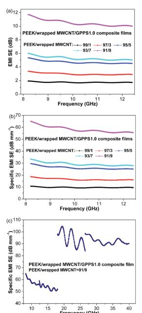
Fig. 5 (a) EMI SE and (b) specific EMI SE for PEEK/wrapped MWCNT/GPPS1.0 composite films with different PEEK/wrapped MWCNT proportion at frequencies of 8.2–12.4 GHz. (c) Specific EMI SE of PEEK/wrapped MWCNT/GPPS1.0 composite films (9 wt% wrapped MWCNT) in four frequency ranges of 8.2–12.4 GHz (X band), 12.4–18 GHz (Ku band), 18–26.5 GHz (K band), and 26.5–40 GHz (Ka band).
