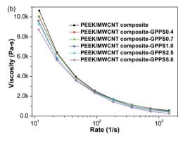
Fig. 1 (a) Dependence of AC conductivity of PEEK/MWCNT composite-GPPSx on frequency at room temperature. (b) Dependence of shear viscosity of PEEK/MWCNT composite-GPPSx on shear rate at 400°
