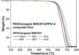
Fig. 4 (a) Electrical conductivities on frequency and (b) TGA curves of PEEK/wrapped MWCNT/GPPS1.0 composite films with different PEEK/ wrapped MWCNT proportion.
