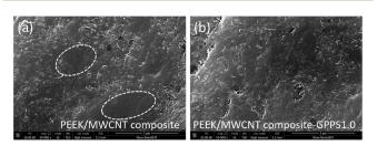
Fig. 2 SEM image of cross-section surface of (a) PEEK/MWCNT composite and (b) PEEK/MWCNT composite-GPPS1.0 (scale bar  $=3\,$   $\mu m).$
