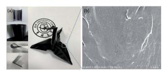
Fig. 6 (a) Digital photographs of a PEEK/wrapped MWCNT/GPPS1.0 composite film with excellent flexibility, *i.e.*, round into a roll, under bending condition and fold into paper crane shape. (b) Cross-section SEM image of composite film.
