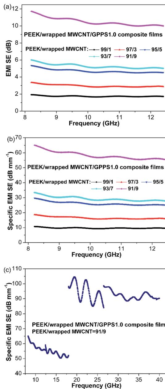
**Fig. 5** (a) EMI SE and (b) specific EMI SE for PEEK/wrapped MWCNT/GPPS1.0 composite films with different PEEK/wrapped MWCNT proportion at frequencies of 8.2–12.4 GHz. (c) Specific EMI SE of PEEK/wrapped MWCNT/GPPS1.0 composite films (9 wt% wrapped MWCNT) in four frequency ranges of 8.2–12.4 GHz (X band), 12.4–18 GHz (Ku band), 18–26.5 GHz (K band), and 26.5–40 GHz (Ka band).
