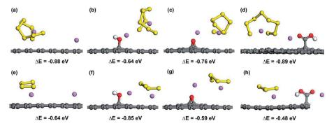
Fig. 7 Atomic configurations and  $\Delta E$  values of Li + LiS<sub>8</sub> and Li + LiS<sub>4</sub> clusters adsorbed on graphene (a and e), hG (b and f), eG (c and g) and cG (d and h) respectively.
