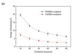
Fig. 3 (a) Efficiency of air aeration and surface discharge-induced calcium sulfite oxidation. (b) Generation efficiency of ozone by PSDBD and LSDBD. (c) Energy utilization of calcium sulfite oxidation by PSDBD and LSDBD.
