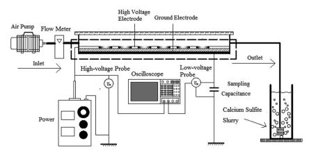
Fig. 1 The schematic of the experimental system.
