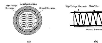
Fig. 2 The schematic of the experimental system: (a) the PSDBD reactor and (b) LSDBD reactor.
