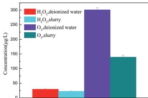
Fig. 10 The variation of O<sub>3</sub> and H<sub>2</sub>O<sub>2</sub> concentration in deionized water and slurry.
