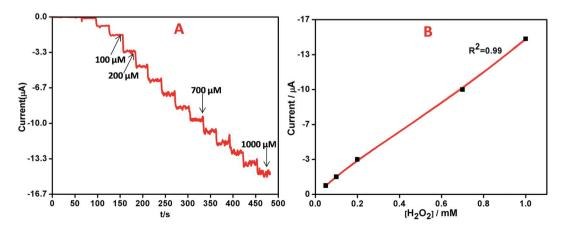
Fig. 10 (A) Amperometric response of AgNPs-rGO-PANI-GCE on increasing the concentrations of  $H_2O_2$  by 0.01, 0.02, 0.05, 0.1, 0.2, 0.5, 1, 2, 5, 10, 20, 50, 100, 200, 500, 1000  $\mu$ M in 0.1 M PBS, pH 7.0 at -0.4 V vs. SCE, (B) the corresponding calibration curves for  $H_2O_2$  analysis.
