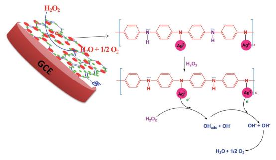
Scheme 2 Schematic representation of the mechanism of H<sub>2</sub>O<sub>2</sub> reduction.
