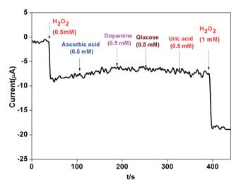
Fig. 11 The amperometric response of AgNPs-rGO-PANI-GC electrode towards  $\rm H_2O_2$  and various interferential compounds (ascorbic acid, dopamine and glucose) in 0.1 M phosphate buffer (pH 7  $\rm \Omega$ )
