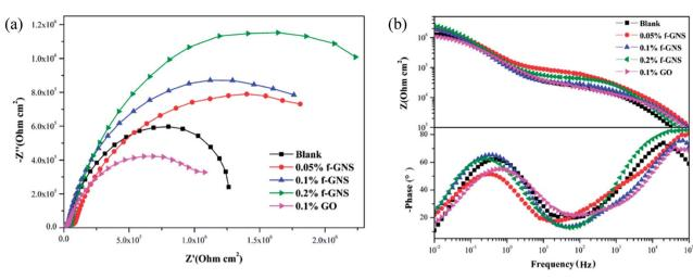
Fig. 10 EIS curves for the silica sol-gel coatings without/with raw and f-GNs nanoplates at the beginning immersion in 3.5% wt% NaCl solution: (a) Nyquist plots and (b) Bode plots.
