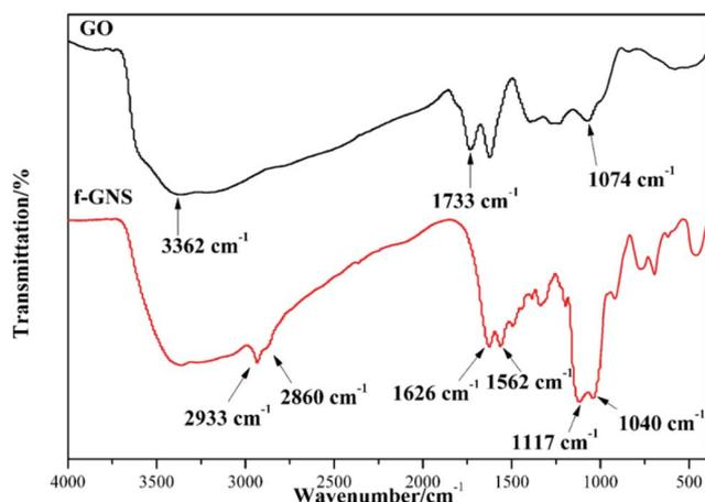
Fig. 1 FTIR spectra of the GO and f-GNs.
