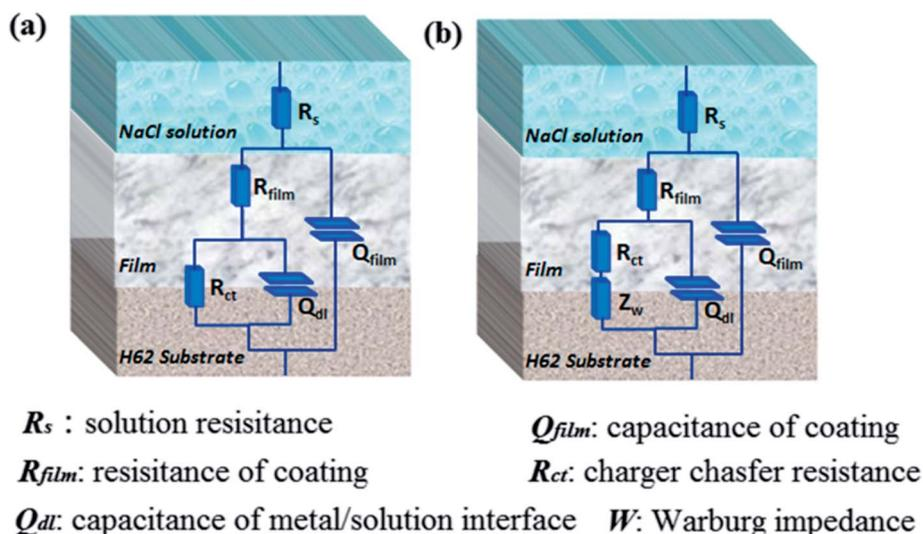
Fig. 13 Equivalent circuits are used to analyze the EIS plots: (a)  $R(Q(R(QR)))$ , used for silica sol-gel coatings without/with f-GNs nanoplates and (b)  $R(Q(R(QRW)))$ , used for silica sol-gel coatings with raw GO.
