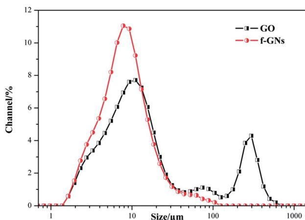
Fig. 7 Diffraction particle size of GO and f-GNs in the silica hybrid sol.
