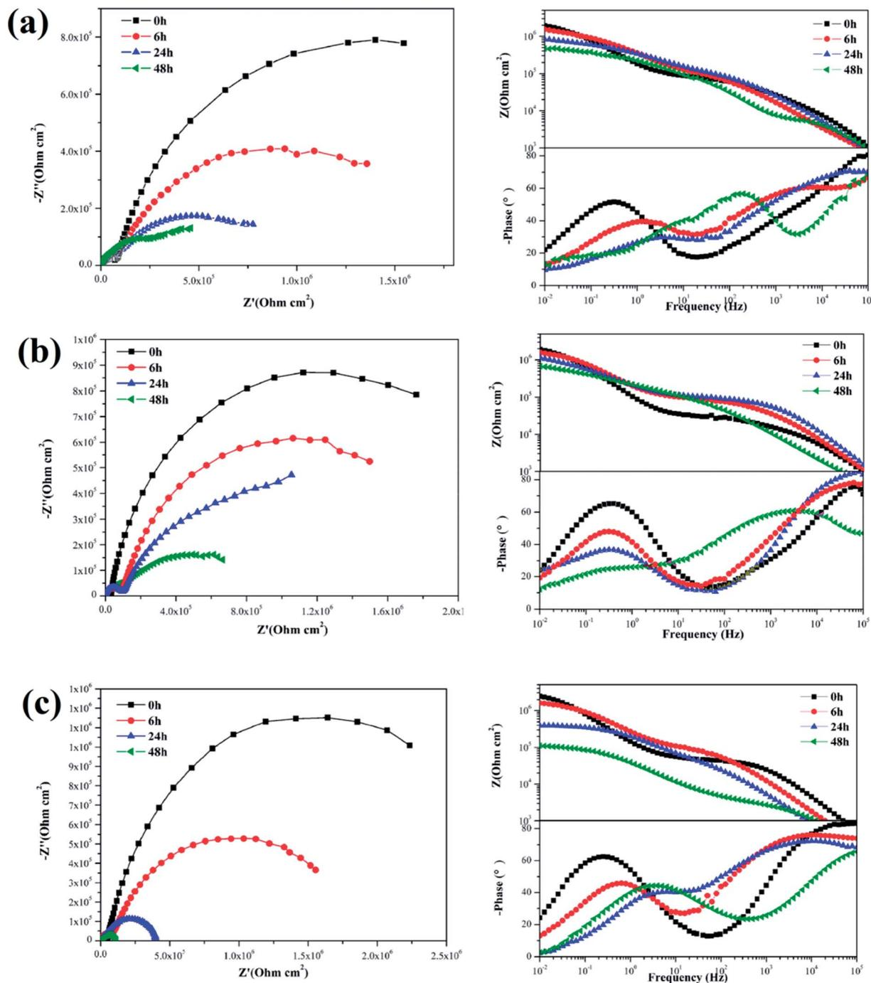
Fig. 12 EIS of silica sol-gel coatings with (a) 0.05% f-GNs, (b) 0.1% f-GNs, (c) 0.2% f-GNs nanoplates different immersion times in 3.5 wt% NaCl solution.
