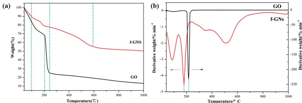
Fig. 5 (a) TGA profiles and (b) DTGA profiles for GO, f-GNS under nitrogen atmosphere.
