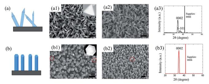
Fig. 1 The schematic crystal models (a and b). Top (a1 and b1) and tilted view (a2 and b2) SEM images, and XRD patterns (a3 and b3) of the GaN NWs grown on c-plane sapphire with GaCl precursor flow rate to be: (a) 9 sccm (b) 16 sccm. The insets a1 and b1 present the cross-section of the NWs. Red circles in b1 and b2 show kinked structures.
