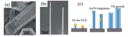
Fig. 4 (a) Ga-droplet on NWs tip by not introducing  $NH_3$  gas during the cooling down process. (b) Au/Ni seed migration on the NW sidewall. (c) The growth process of thick GaN NWs including Ni/Au-catalyzed growth, Au/Ni migration and consumption, Ga-catalyzed growth.
