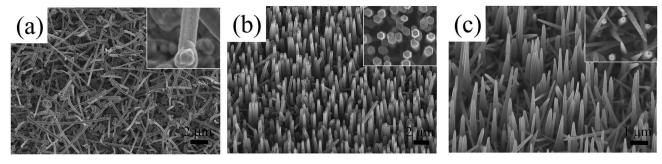
Fig. 3 The effect of metal catalyst thickness on GaN NWs growth on *c*-plane sapphire: (a) and (b) SEM images of GaN NWs grown on: 4 nm Ni/Au with GaCl flow 9 sccm and 16 sccm, respectively. (c) and (d) SEM images and TEM images of GaN NWs grown on 8 nm Ni/Au with GaCl flow 16 sccm. Inset of the pictures show the cross section of GaN NWs.
