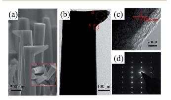
Fig. 5 GaN NW crystallographic orientation transition during growth: (a) side-view SEM image of kinked NW structures grown on c-plane sapphire. (b)-(d) Low and high magnification TEM images and SAED pattern illustrating growth direction switching. The inset (a) presents the tilted view of a kinked NW. The SAED pattern confirms the branch NWs are homoepitaxial grown on the stand rod.
