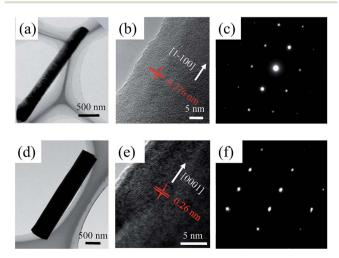
Fig. 2 TEM images of m- and c-axis GaN NWs, which is obtained with GaCl flow of (a)–(c) 9 sccm, (d)–(f) 16 sccm respectively. Low- and high-magnification TEM is shown in a, d and b, e. The corresponding SAED is shown in c and f.
