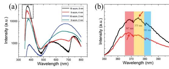
Fig. 6 Photoluminescence (PL) measurements of different crystallographic orientation GaN NWs grown on c-plane sapphire: (a) under GaCl flow of 9 sccm (blue, Au/Ni: 1/1 nm), 9 sccm (red, Au/Ni: 2/2 nm), 16 sccm (gray, Au/Ni: 1/1 nm), 16 sccm (black, Au/Ni: 4/4 nm); (b) a highresolution PL spectrum of the dotted box area in (a) in a linear scale.
