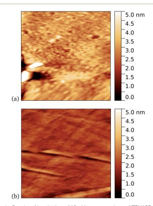
Fig. 6 Results of incubation of 10 nM concentrations of TEM105-azF molecules with graphene for 10 minutes (a) with UV illumination, 0.6  $\mu$ m AFM image and (b) in the dark, followed by a 1 minute rinse, 1  $\mu$ m AFM image. Regions of high coverage are found for UV but not for the dark.
