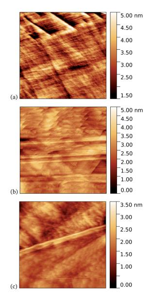
Fig. 10 STM images. (a) A 1.1  $\mu$ m square image of pristine graphene. After incubation of 10 nM concentration of cyt  $b_{562}$ -azF molecules with graphene for 10 minutes (b) in dark, 0.9  $\mu$ m square and (c) with UV illumination, 0.4  $\mu$ m square.
