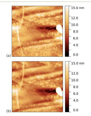
Fig. 9 Results of incubation of 5 nM concentrations of cyt  $b_{562}$ -azF molecules with graphene for 10 minutes with UV illumination, then rinsed for 15 minutes. AFM images of 0.59  $\mu$ m squares show the proteins are robust to multiple scans. (a) 1st scan of area, (b) 10th scan. The heights of the proteins are around 2 nm.
