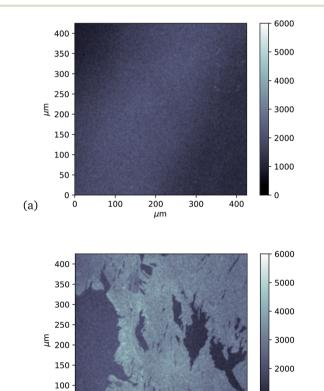
Fig. 5 Approximately 400  $\mu m$  square confocal microscopy images to compare fluorescence from separate single-layer graphene on silicon samples incubated with GFP204-azF molecules (10 nM) (a) in the dark and (b) with 10 minute UV exposure, each followed by thorough rinsing with deionised water for one minute. (The vertical intensity scale is arbitrary and the same for each sample.) Images taken using a Zeiss LSM880 confocal laser scanning microscope.
