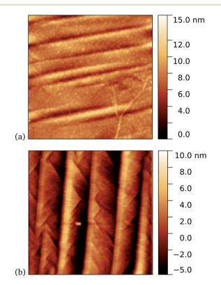
Fig. 8 Results of incubation of 5 nM concentrations of Cyt b<sub>562</sub>-azF molecules with graphene for 10 minutes (a) with UV illumination and (b) in the dark, followed by a 5 minute rinse. AFM images of 1  $\mu$ m square show regions of high coverage for UV but generally much less for the dark
