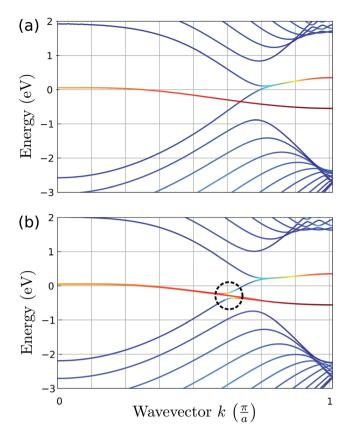
Fig. 3 Band structure of a flat GNR (a) and a bent GNR, with the curvature radius R=0.5 nm (b). The reddish bands are derived from the edges of the ribbon, the blue bands do not have a projection on the edges and intermediate colors apply for mixed states.
