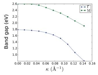
Fig. 6 Electronic band gap at the  $\Gamma$  and M points as a function of curvature. The system band gap is always located at  $\Gamma$ ; the band gap at M is just a parameter to quantify bending effects. Surface states were ignored in the gap measurement.
