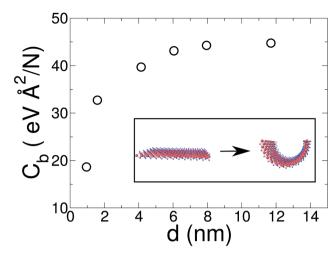
Fig. 4 Bending modulus of a  $MoS_2$  ribbon as a function of its width d. MO: blue; S: red.
