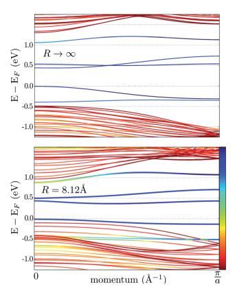
Fig. 5 Band structure of an armchair  $MoS_2$  nanoribbon. The upper and lower panels correspond to a flat  $(R \to \infty)$  and a bent nanoribbon, respectively. The color code shows the (real-space) localization of the eigenvalues: red is used for the inner subbands (i.e. bulk-like), while the edge subbands are blue; intermediate colors correspond to the hybridization of bulk and edge states.
