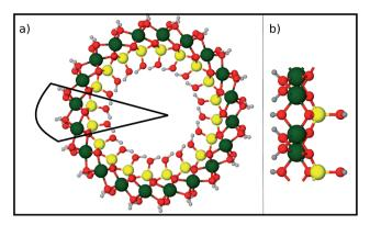
Fig. 7 Structure of an imogolite nanotube. (a) An axial view of imogolite for  $N_{\theta}=10$ . The basic unit is marked by the continuous black line. (b) A side view of the basic imogolite unit [(OH)<sub>3</sub>Al<sub>2</sub>O<sub>3</sub>SiOH]<sub>2</sub>, that is repeated  $N_{\theta}$  times to form the nanotube. Green Al; red O; yellow Si; and light gray H.
