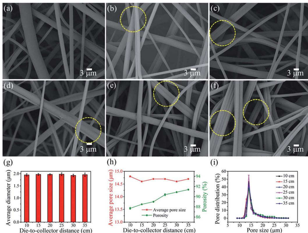
Fig. 2 Morphology and pore structure of PP melt blown nonwovens. SEM images of PP melt blown fabricated at DCD of (a) 10, (b) 15, (c) 20, (d) 25, (e) 30 and (f) 35 cm. (g) Average diameter, (h) average pore size and porosity, (i) pore size distribution.
