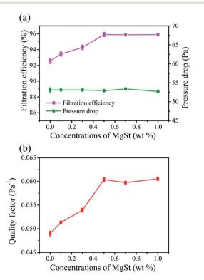
Fig. 5 Filtration performance of the charged PP/MgSt melt blown nonwovens. (a) Filtration efficiency and pressure drop and (b) quality factor value.
